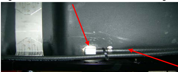
Figure 3. 1/2" STOR x 3/8" hose barb 90 degree tank fitting
