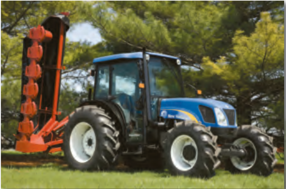
Disc Mowers Disc mowers cut by the slicing rather than shear cutting and mow more quickly than sickle bar mowers; they can handle fine grasses with wet or dead undergrowth and effortlessly cut through ant hills.
