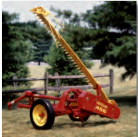
Sickle Bar Mowers Simplicity, high speeds, and greater widths keep the sickle bar mower popular. Forged steel cutterbar guards penetrate fine grasses and dense undergrowth with ease.
