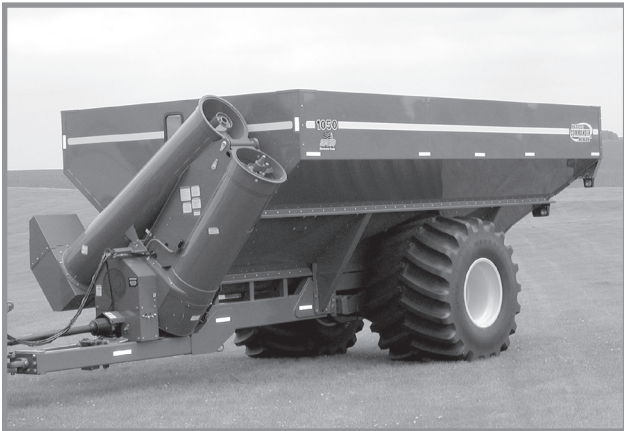
Model 1050 Sof-Tred Wagon Shown With Vertical Auger In Storage/Transport Folded Position
