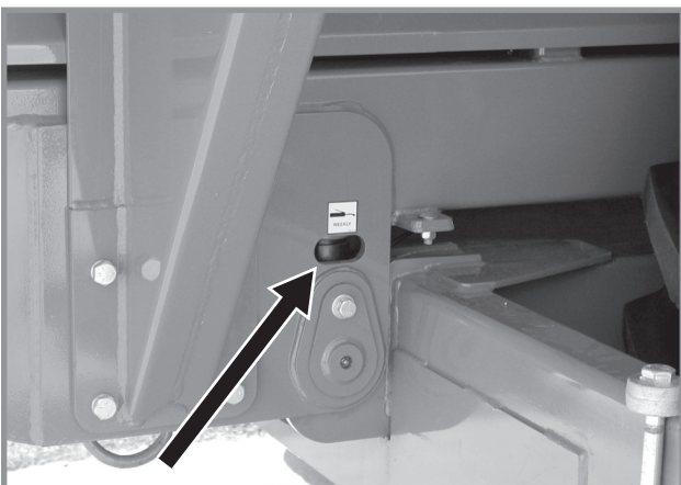
1050 Compression Type Load Cell
