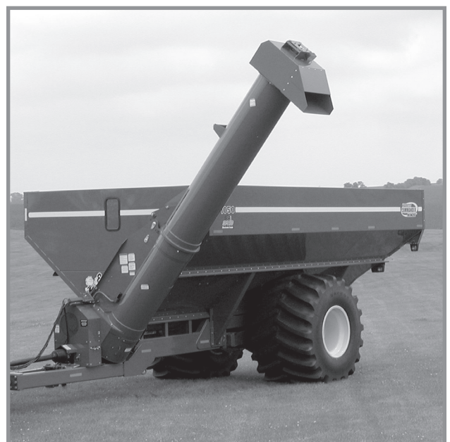
Model 1050 Sof-Tred Wagon Shown With Vertical Auger In Unloading Position
