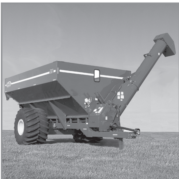
Model 850 Sof-Tred Wagon Shown With Vertical Auger In Unloading Position
