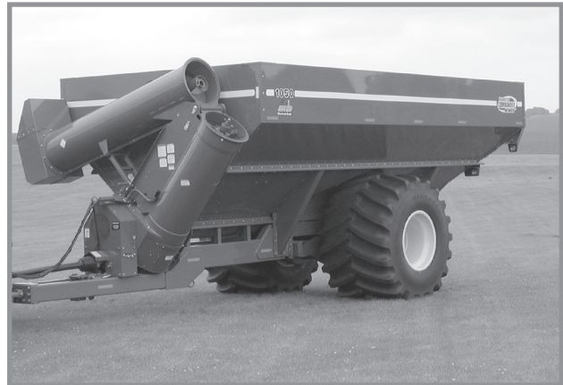
Model 1050 Sof-Tred Wagon Shown With Vertical Auger In Field Folded Position
