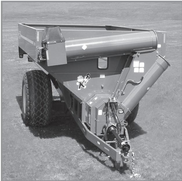
Model 650 Wagon Shown With Vertical Auger In Transport/Field Folded Position
