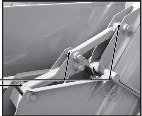
Fold Linkage And Hinge (4 Zerks)
