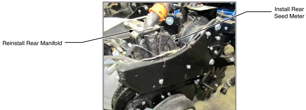
Rear Meter and Manifold Shown Installed
