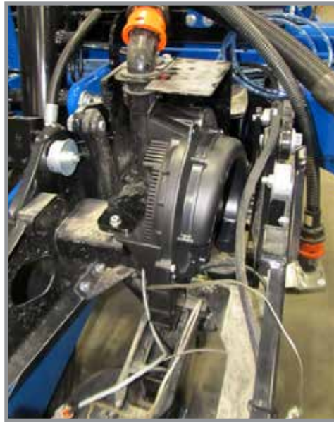
Front Meter and Manifold Shown Installed
