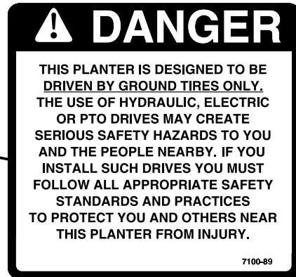
Part No. G7100-89 (Qty. 2 - One Located At End Seed Rate Transmission On Each Side Of Planter)
