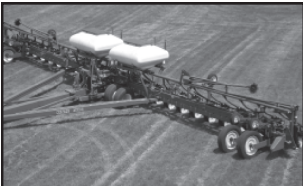
24 Row 30" SDS Machine Shown In Field Operation Position
