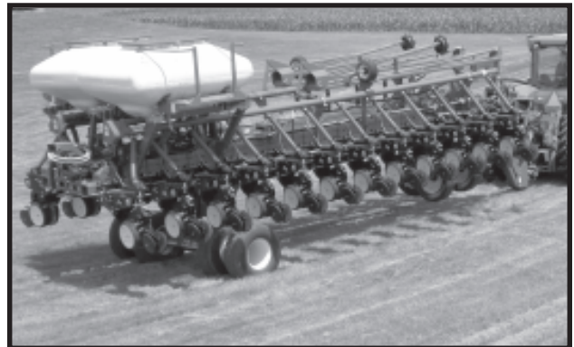
24 Row 30" SDS Machine Shown In Transport Position
