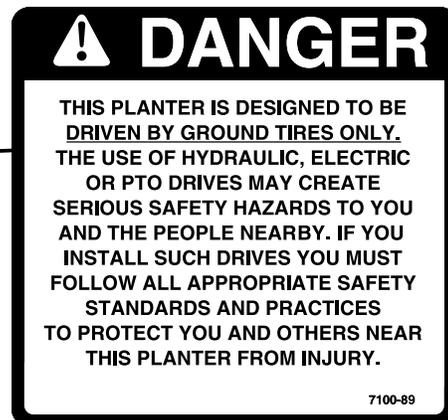
Part No. G7100-89 (Qty. 2 - Located On Wheel Modules On Both Ends Of Planter)
