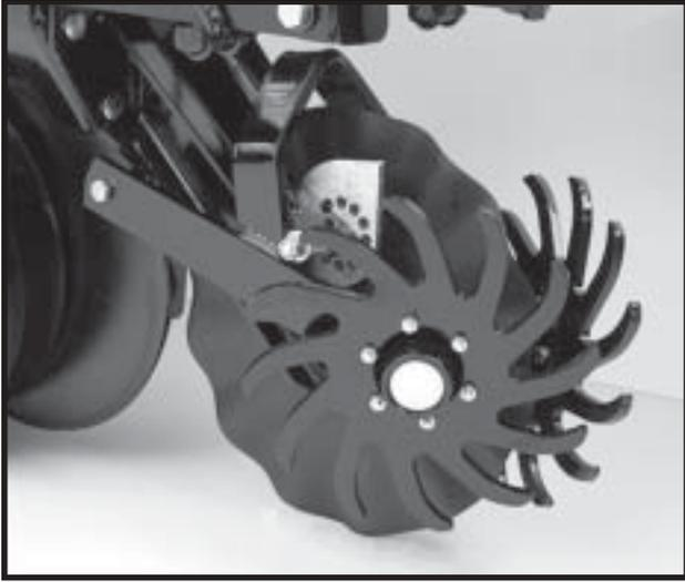
The wheel hubs are equipped with sealed bearings. If bearings sound or feel rough when the wheel is rotated, replace the bearings.
