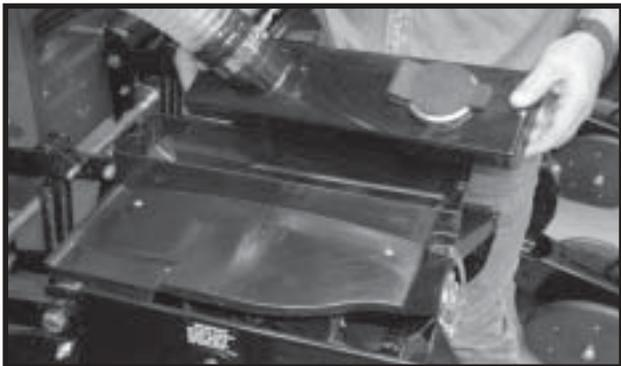
Disengage the seed drive and remove the seed mini-hopper and meter.
