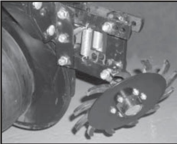
The wheel hub is equipped with sealed bearings. If bearings sound or feel rough when the wheel is rotated, replace the bearings.
