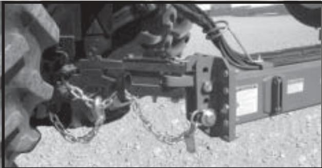
1. Adjust tractor drawbar to 13-17 inches above the ground. Adjust the drawbar so the hitch pin hole is directly below the center line of the PTO shaft. Make sure the drawbar is in a stationary position. See page 6-14 when using the even-row push row unit option.
