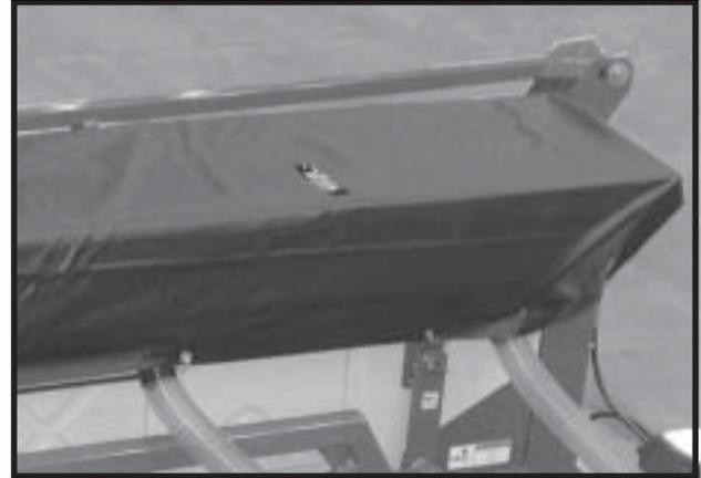
**NOTE:** The bulk seed hoppers are not water tight. Store the planter inside when possible. Fitted covers, for use if the planter must be stored outside, are available from KINZE® Repair Parts. Secure covers using grommets in covers and customer-supplied rubber tarp straps as needed.
