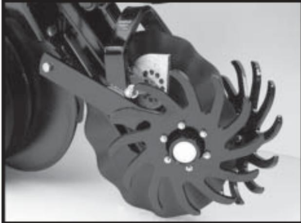
Coultter mounted residue wheels are designed for use on pull row units and push row units.
