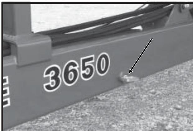
8. Install transport latch locking pin.
