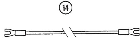
Jumper Wire Between Terminal Strips On Valve Block On Rear Center Frame (See Pages P92 And P93)
