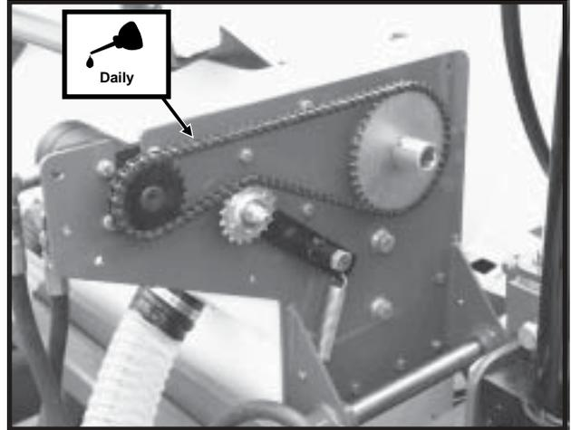
**Bulk Fill System Hydraulic Motor Chains**
