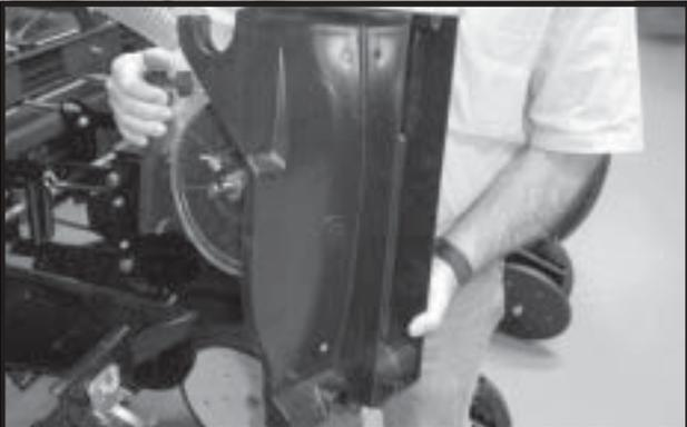
Remove seed disc by loosening wing nuts. Empty the meter. Thoroughly inspect brushes to ensure all seed is removed. Replace seed disc and install wing nuts.
