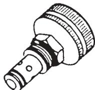
The flow control valves should be adjusted for row marker raise and lower speed as part of the assembly procedure or upon initial operation. If the valve fails to function properly or requires frequent adjustment, it should be removed for inspection. Check for foreign material and contamination on both the valve and the seating area of the valve body. Replace any components found to be defective.
