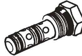
The pilot operated check valve prevents the wing lock cylinders from retracting without applied hydraulic pressure. The wing lock cylinders become the wing flex upper stop during field operation. If the valve fails to function properly, remove the valve from the valve block and check for foreign material or check to see if the o-ring is leaking internally. Replace if found to be defective.
