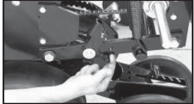
4. Using the lift lever, raise the push row unit to allow the spring loaded lockups to snap into locked position under the row unit stops.
