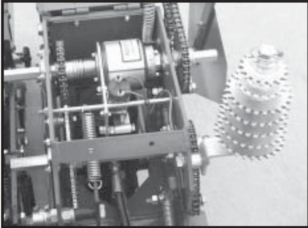
The point row clutches are permanently lubricated and sealed and require no periodic maintenance. **DO NOT LUBRICATE. KEEP CLUTCHES CLEAN.**
