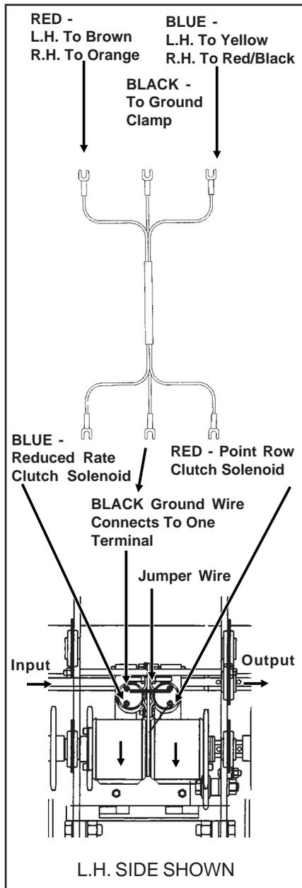
**NOTE:** Before doing any electrical work, disconnect the control console from the tractor battery. Keep wiring harnesses away from high temperature areas or sharp edges. DO NOT route the wiring harnesses along battery cables. Use tie straps to keep wire harness away from moving parts on tractor and planter. Be sure ground connections to the tractor frame are clean to provide good electrical contact.
