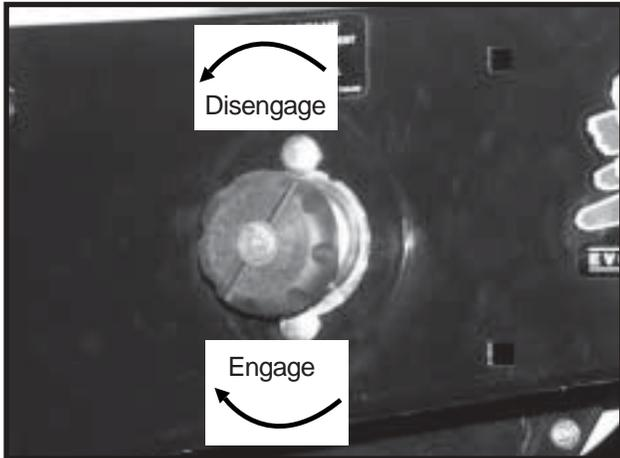
To disengage the drive, turn the knob  $\frac{1}{4}$  turn counter-clockwise. To engage the drive, turn the knob  $\frac{1}{4}$  turn clockwise.
