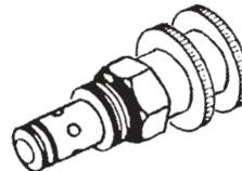
The flow control valve allows auger speed to be varied to meet seed demand. If the valve fails to function properly or requires frequent adjustment, it should be removed for inspection. Check for foreign material and contamination on both the valve and the seating area of the valve body. Replace any components found to be defective.
