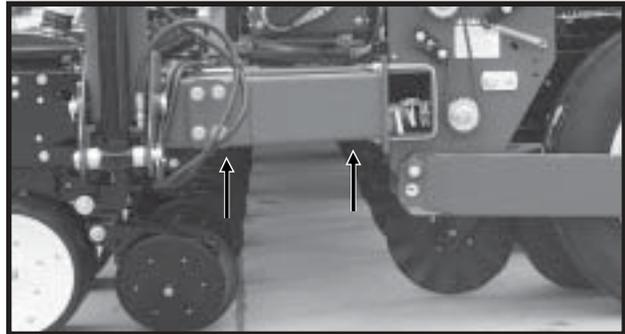
With the planter lowered to proper operating height, check to be sure the frame is level fore and aft. Recheck once planter is in the field.
