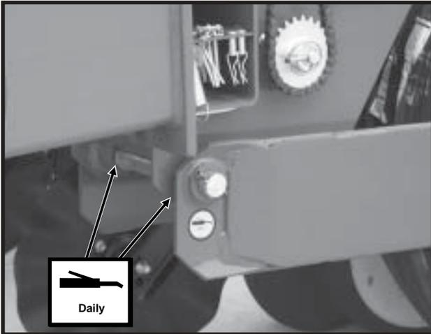
2. Wing Wheel Pivot - 2 Zerks Per Wheel Module
