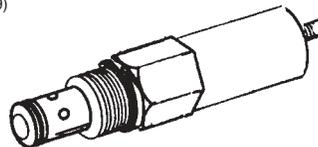
If the pressure relief valve fails to release the tongue lock or function properly, remove the valve from the valve block and check for foreign material or check to see if the o-ring is leaking internally. Replace if found to be defective.
