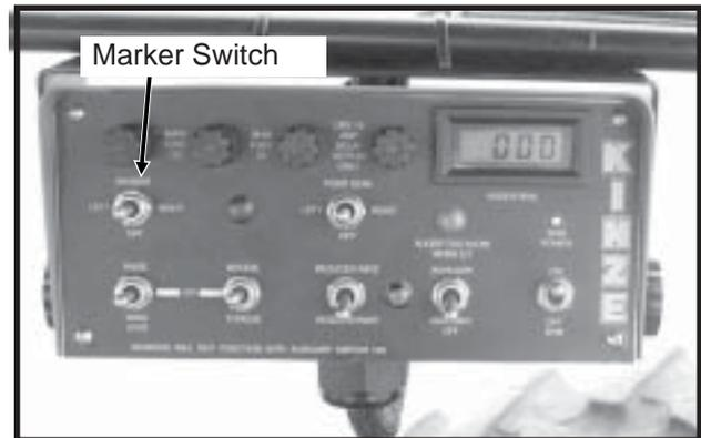
Three Position Selector Switch On Bulk Fill Planter Control Console
