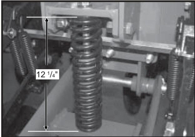
**NOTE:** The piston pump ground drive wheel assembly is designed to allow the assembly to be locked in raised position when not in use. Remove the two cap screws that attach the upper end of the spring to the spring mount. Reattach the spring using the upper holes in the spring mount. Reverse procedure to reset for field use.
