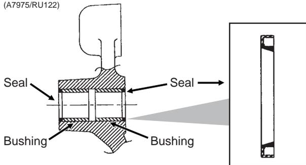
4. Drive/press replacement bushing inside bore of arm to a depth of .125" below flush.
