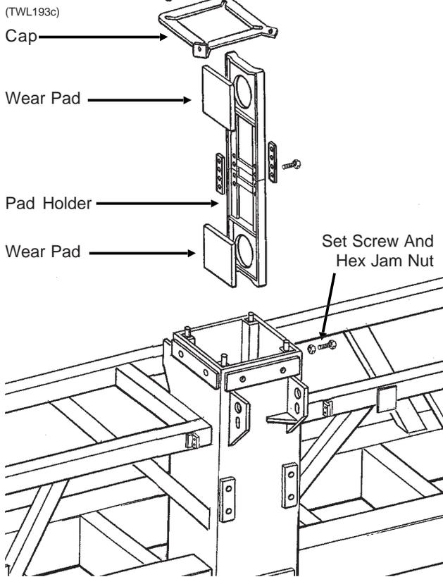
The center section of the planter consists of a steel tubular frame equipped with four wear pad assemblies which travel up and down against a stainless steel clad center post. Each wear pad assembly consists of a pad holder and two wear pads. The wear pads are held in place by the pad holder and adjusted and locked in adjustment by  $\frac{3}{4}$ " set screws and hex jam nuts.
