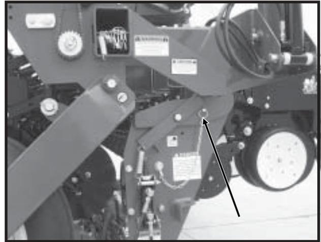
9. Remove manual safety lockup from its storage location on the hose take-up on the planter hitch and position it behind the front center lift cylinder.
