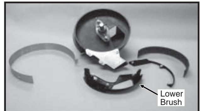
The lower brush has several functions. One function is to move seed down the seed loading slots to the seed pockets. The second function is to isolate seed in the reservoir from entering the seed tube and a third is to clean the seed loading slots.
