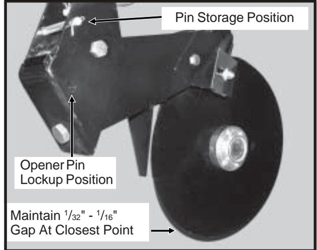
The outer scrapers on each disc blade may also be adjusted to make up for wear that may occur. Make sure the scrapers are adjusted to allow only slight contact with the blades.
