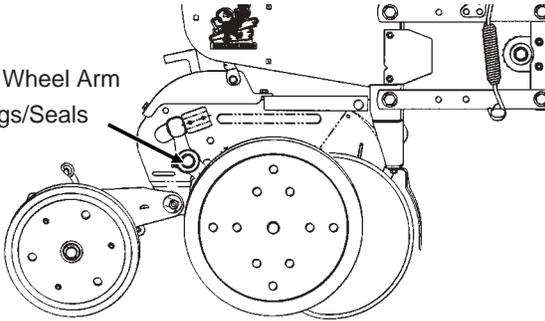
**NOTE: A Gauge Wheel Arm Bushing And Seal Driver Kit (G1K296), for use in bushing and seal replacement, is available through your KINZE® Dealer.**
