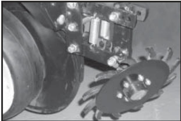
Two adjustable springs on the parallel links on each residue wheel allow for down force adjustment. Position 1 as shown at right provides minimum down pressure and position 3 maximum down pressure.
