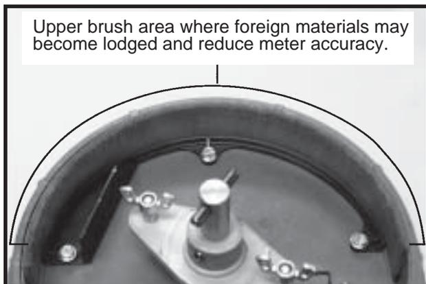
**IMPORTANT:** Close bulk seed hopper lids after hoppers are filled to prevent accumulation of dust or dirt in the seed meter which will cause premature wear.
