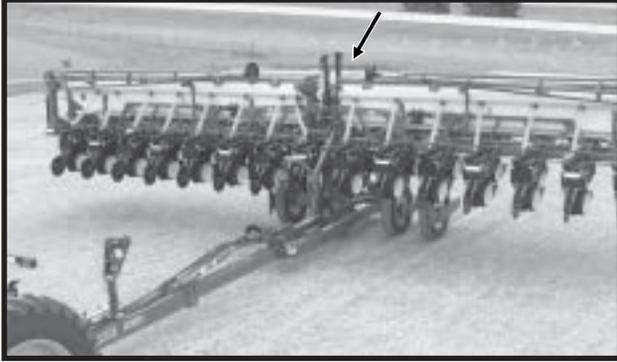
6. Hold the control console switch labeled "ROTATE/TONGUE" in "ROTATE" and operate the hydraulic lever to rotate the planter until the transport latch is engaged.
