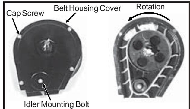
If the belt is being replaced, make sure it is installed to correctly orient the paddles as shown. A diagram molded into the drive sprocket also illustrates the correct orientation.
