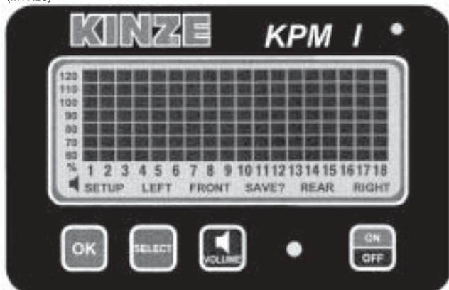
The electronic seed monitor system consists of a console, which is mounted on the tractor; seed tubes with computerized sensors, one of which is installed in each planter row unit; a primary harness\*, which connects the console to the planter harness; and a planter harness (junction Y-harness and/or harness extension where applicable), to which the individual seed tube sensors connect.
