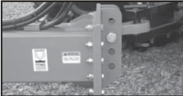
Four holes in the hitch bracket allow the clevis to be raised or lowered. In addition, the clevis may be turned over for a finer adjustment between mounting holes. When installing the clevis mounting bolt, make sure the lock nut is tightened to proper torque setting.
