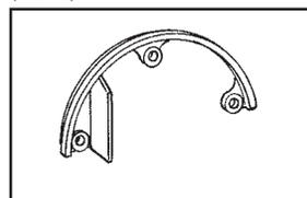
Use GD11122 upper brush retainer when using soybean and cotton discs.
