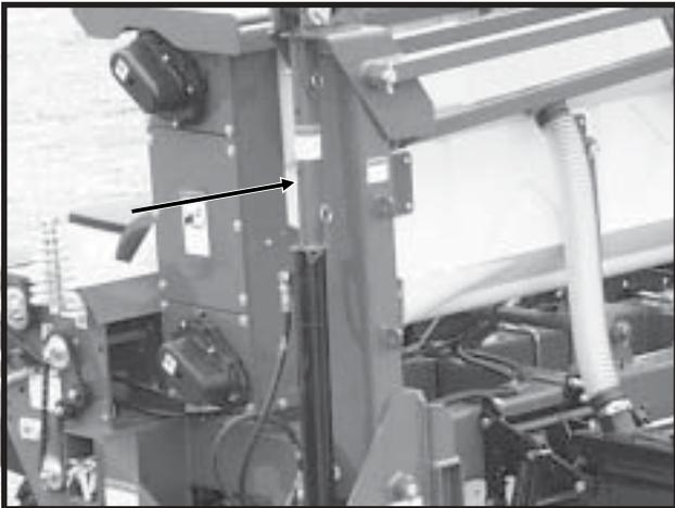
2. Using the hydraulic lever, raise the planter to the raised field position as shown below.
