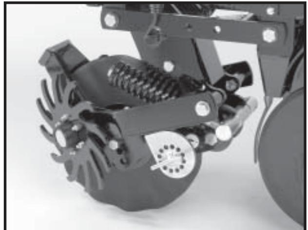
The wheel hub is equipped with sealed bearings. If bearings sound or feel rough when the wheel is rotated, replace the bearings.
