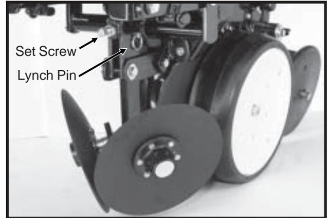
Vertical adjustment in  $\frac{1}{3}$ " increments is possible by removing the lynch pin which secures the vertical support arm and moving the support arm up or down as required. Re-install lynch pin. Finer adjustment can be attained by removing the lynch pin and using the  $\frac{5}{8}$ " x  $2 \frac{1}{4}$ " set screw to clamp the support arm in the required position.
