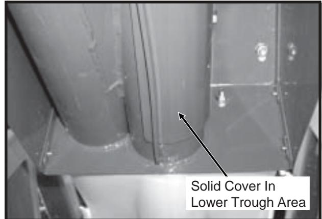
Two covers are provided for the lower auger trough. A mesh screen is used for most larger seeds, including corn and soybeans. A solid cover, to replace the screen, is supplied with the planter for use when planting very small seeds.
