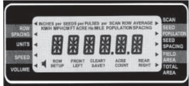
Press the UP or DOWN arrow keys to move the flashing arrow on the lower LCD to change what is displayed on the lower LCD.
