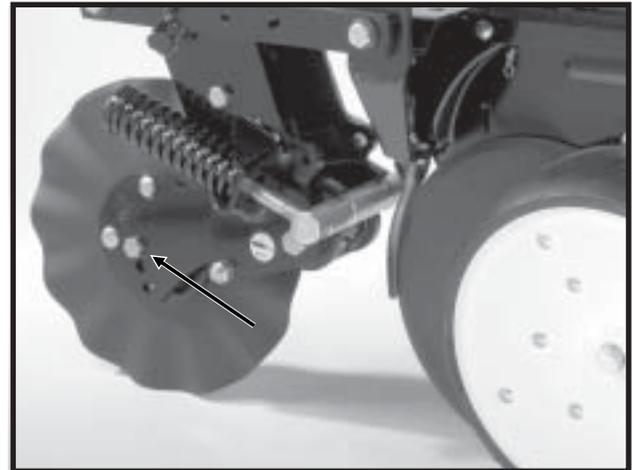
**NOTE:** Torque  $\frac{5}{8}$ " spindle bolts to 120 ft. lbs.
