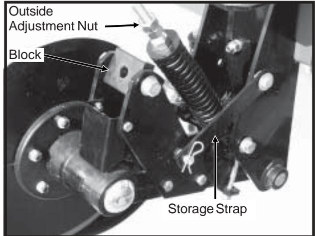
**NOTE: The HD single disc fertilizer opener is equipped with a lockup bar that automatically raises and locks the soil press wheel when the blade assembly is raised.**
