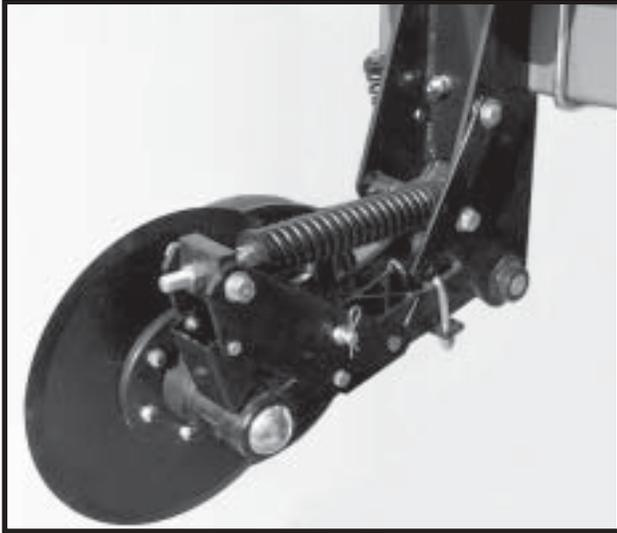
Placement of fertilizer with the HD single disc fertilizer opener is recommended at 3 1/2" - 4" from the row. **Never locate the opener to place fertilizer closer than 2".**
