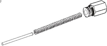
The pressure relief valve limits the applied pressure to the hydraulic auger drive motors to prevent mechanical damage to the motors. If the valve fails to function properly, it should be removed for inspection. Check for foreign material and contamination on both the valve and the seating area of the valve body. Replace any components found to be defective.
