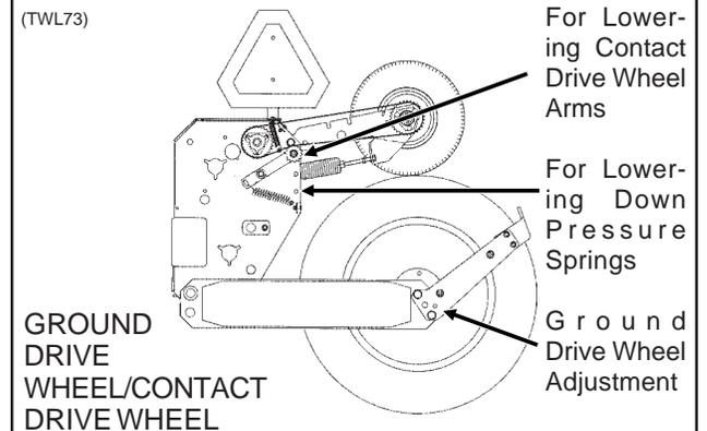
When the planter has been fully loaded with seed, granular chemicals, etc.; a field check should be made to be sure the wings are level with the center frame. If the wings are not level with the center frame, the drive wheels and/or transport wheels can be raised or lowered in the wheel arms to increase or decrease planter toolbar height. Hitch height should be raised accordingly to ensure level operation.
