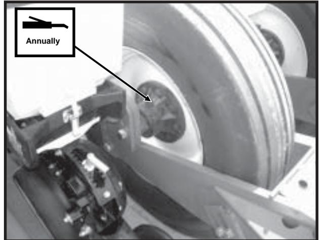
10. Transport Wheel Bearings - 1 Zerk Per Hub
