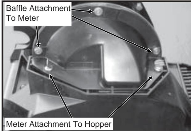
Rotate the seed meter drive by hand to ensure that the springs are holding the tabs of the fingers against the carrier plate where indicated in the photo and that the fingers are being raised in the correct area.
