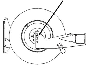
**NOTE: The toolbar should operate at a 20"-22" height measured from the bottom of the toolbar to the planting surface.**
