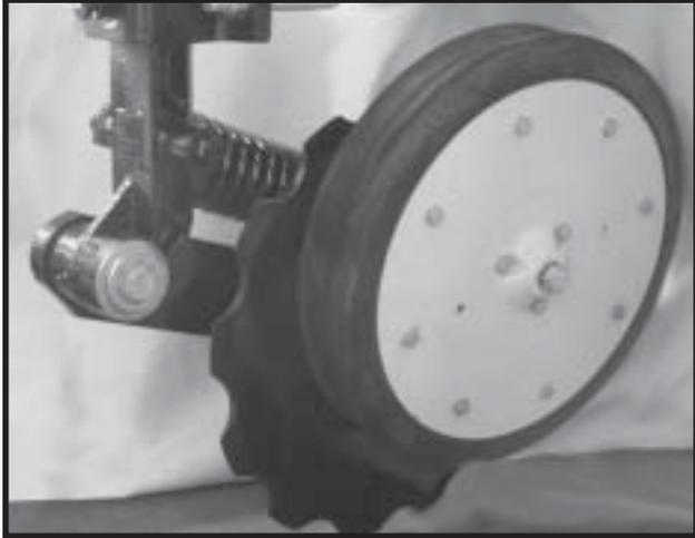
The depth/gauge wheel attachment for the notched single disc fertilizer opener is designed for use in situations where additional gauging is required to maintain desired fertilizer opener depth. The depth/gauge wheel is attached to the notched single disc fertilizer opener using a mounting block fastened to the pivot arm using  $\frac{5}{8}$ " hardware through the disc blade hub w/bearing.
