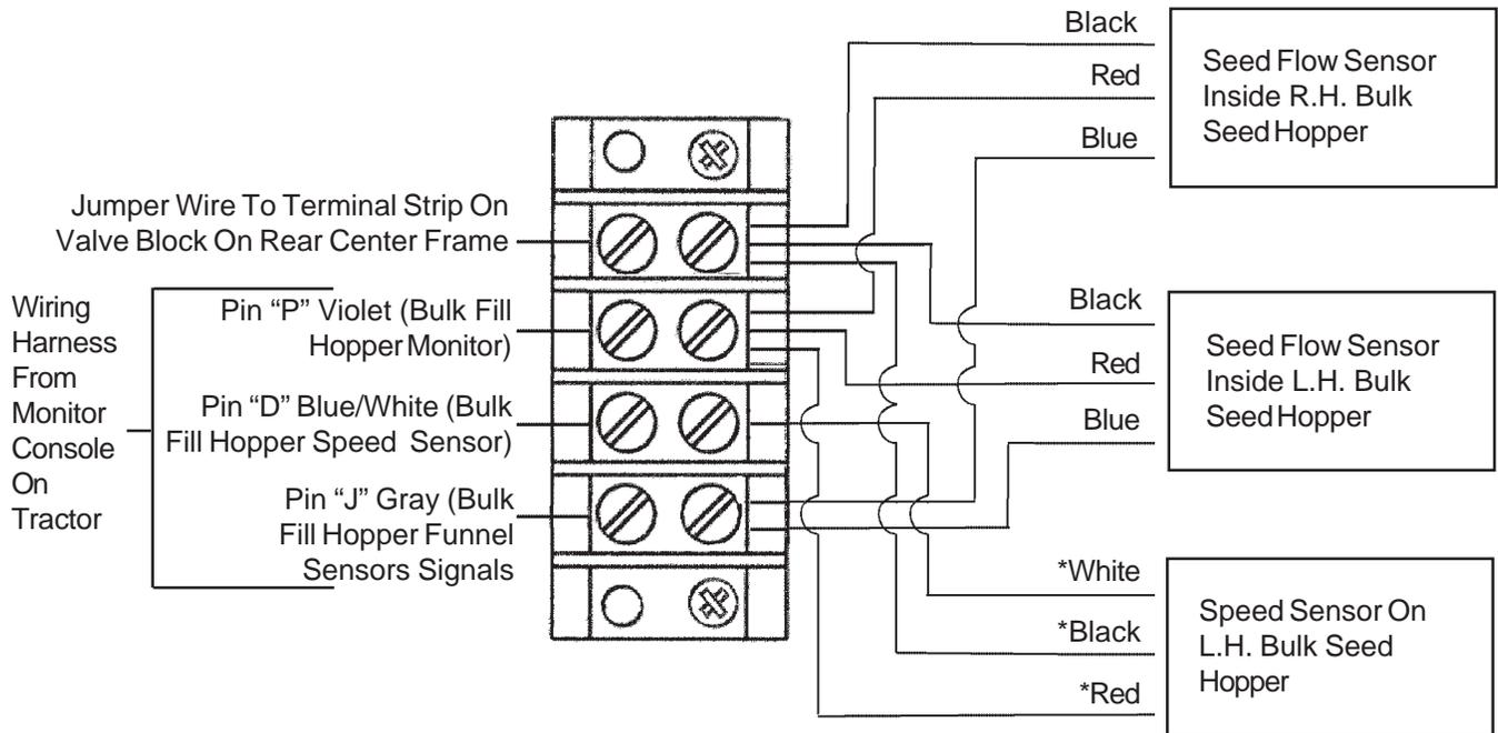
\* Speed Sensor wire colors are identified by heat shrink tape.
