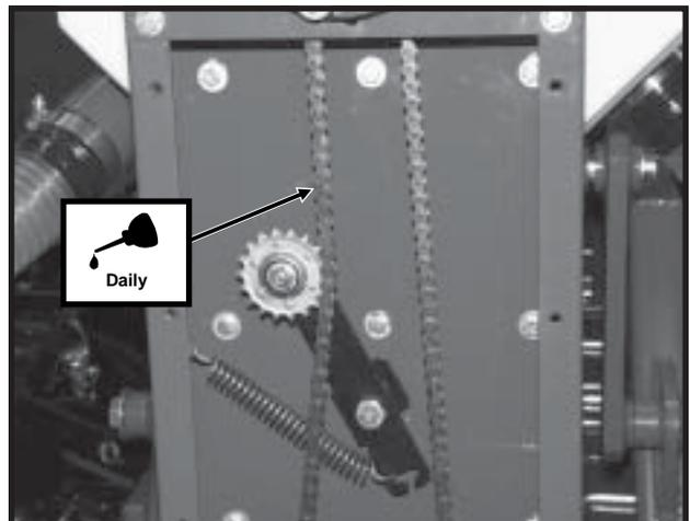
**Bulk Fill System Gearbox Chains**
