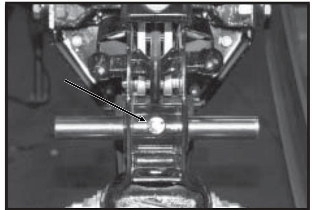
3. Install the replacement spindle and position as shown below. Exact centering is critical.
