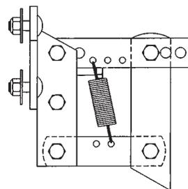
To adjust down force springs, raise the row unit out of the ground and reposition springs as shown for the desired down pressure.
