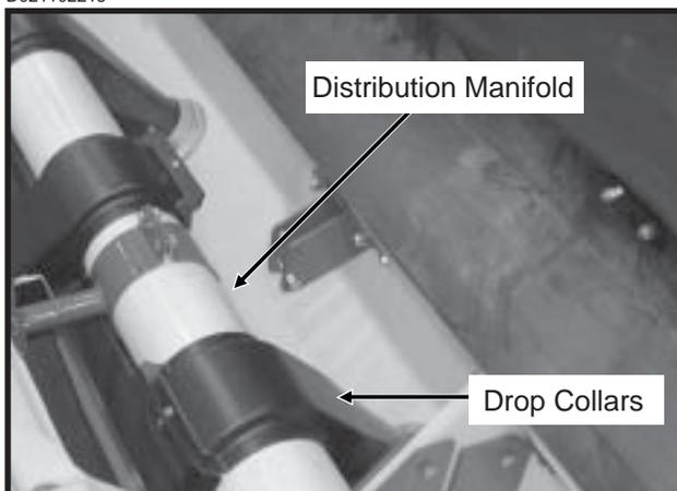
**NOTE:** After all row outlets are filled to capacity, seed will continue to be evenly distributed to all rows until the bulk seed hopper is empty. When the bulk seed hopper is empty or the auger system is shut off, all drop hoses will “plant out” equally and all rows should run out of seed at approximately the same time.
