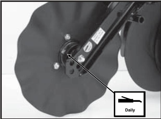
(If Applicable) Row Unit Mounted No Till Coupler Hubs -
