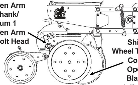
**Shim Gauge Wheel To Lightly Contact The Opener Disc Blade-Check Adjustment In Field Position**
