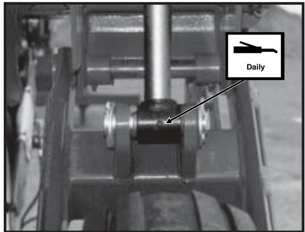
11. Wing Lift Cylinders - 1 Zerk Per Cylinder
