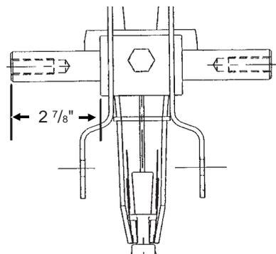
4. Install 1/2" x 3/4" cap screw and torque to lock pivot spindle in place.
