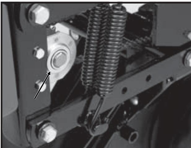
A number of sealed bearings are used on your KINZE® planter to provide trouble free operation. These are located in such areas as the drive shaft, row units and transmission bearings. Sealed bearings are lubricated for life. Due to the seals, relubrication is not practical.
