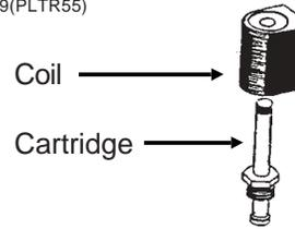
The solenoid valve consists of a chambered body containing a cartridge valve which is activated by an electrical coil.
