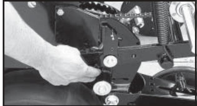
3. Using the lift lever, raise the push row unit to allow the spring loaded lockups to snap out of locked position. Lower row unit to the ground.
