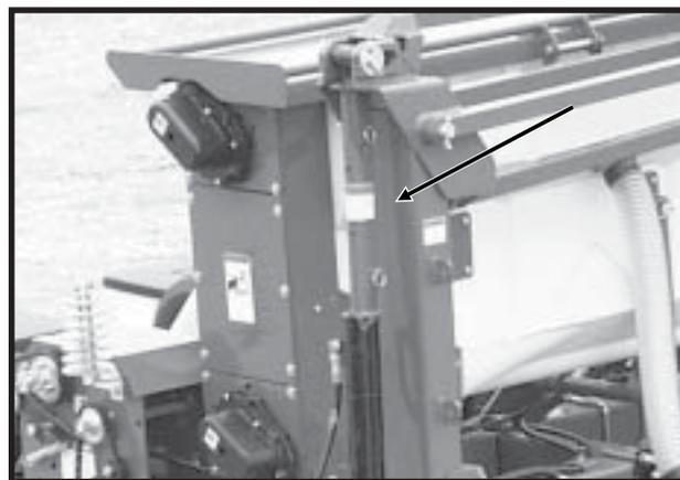
Marker Lockup (Bulk Fill System Shown)
