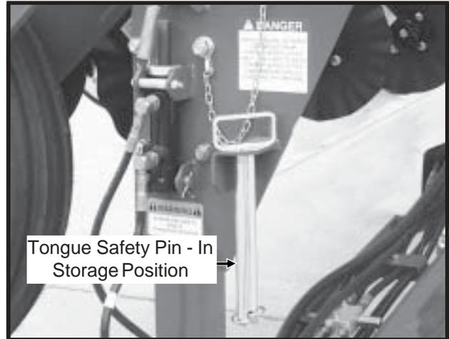
2. Remove the transport latch locking pin from the locked transport position and place it in the storage location.
