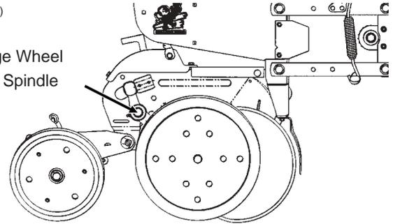
**To replace gauge wheel pivot spindle:**
