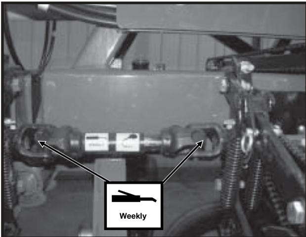
8. U-Joints - 2 Zerks Per Hinge Area
