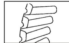
**Hill-drop cotton, acid-delinted:** 12 cells, 3 to 6 seeds/cell, to meter seed sizes from 4000 to 5200 seeds per pound (Brown color-coded).
