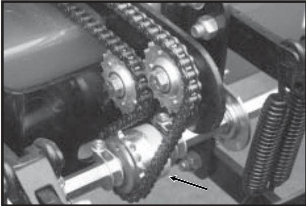
The push row unit clutch sprockets are designed to allow the push row unit drill shafts to be disengaged when only the pull row units are being used.
