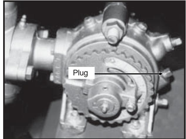
Check crankcase oil daily and maintain at plug level. Fill as needed with EP 90 weight gear oil. Total oil capacity is approximately  $\frac{3}{4}$  pint.
