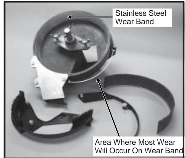
The purpose of the stainless steel wear band is to protect the meter housing from wear. The band is .030" thick and should be replaced when approximately .020" of wear is found in the primary area of wear. If the wear band is allowed to wear through or if the meter is used without the wear band in place, damage to the meter housing may occur.
