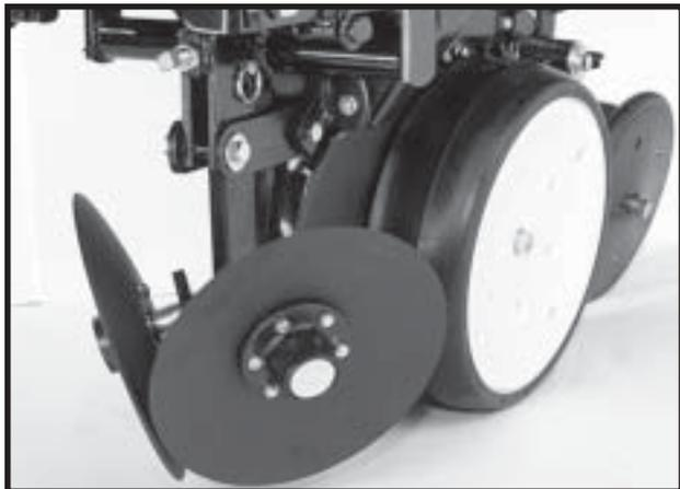
Lubricate the bushings in the support arm and mounting bracket at the frequency indicated in the Lubrication Section of this manual. Using a torque wrench, check each bolt for proper torque. If the bolt is loose, it should be removed and the bushing inspected for cracks and wear. Replace bushings as necessary. **Only hardened flat washers should be used. Replace damaged flat washers with proper part. Torque bolts to 130 ft. lbs.**
