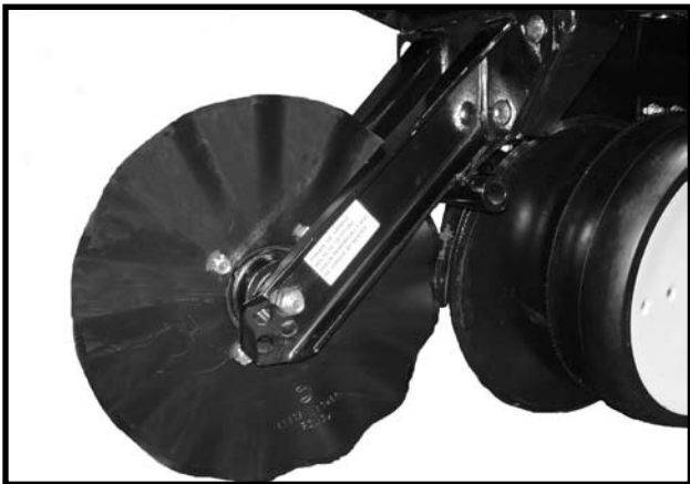
STYLE B (One Sleeve For Installing Coulters Mounted Residue Wheels)
