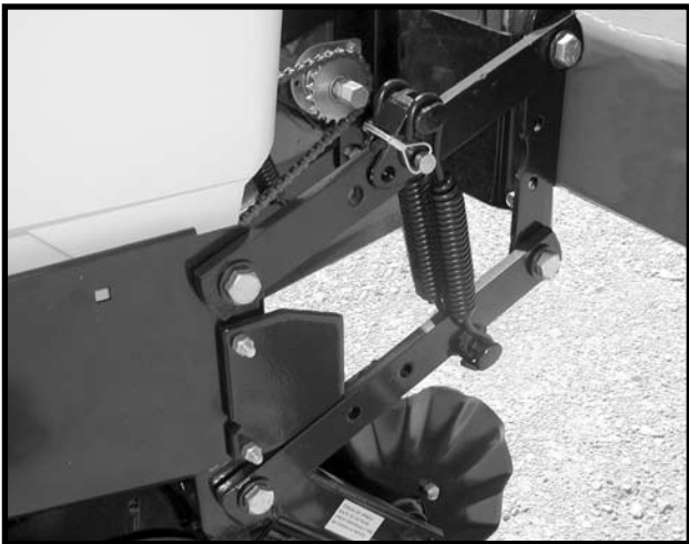
Four Springs Per Row (Quad) (Used Only In Conjunction With Row Unit Mounted No Till Coulters)
