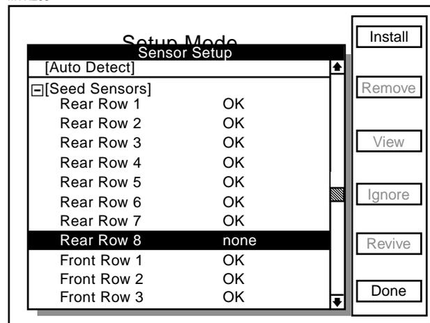
**STEP 6** Unplug the sensor and plug in a new sensor. Press F1 key next to Install.
