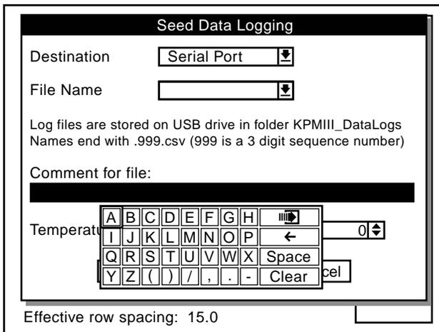
**STEP 7** Use the knob or arrow keys to scroll to the Temperature box. Press the knob or Enter key to display the drop down keyboard. Use the keyboard to enter the temperature then press the Enter key.
