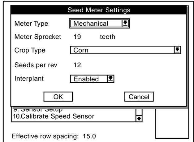
**NOTE:** When Mechanical “Meter Type” is selected “Meter Sprocket” automatically sets.
