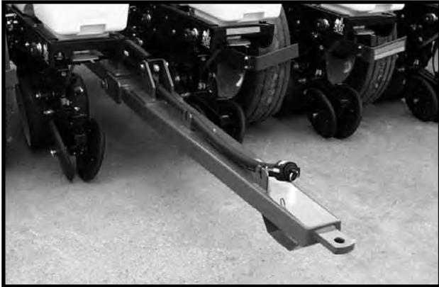
The Rear Trailer Hitch is used to tow a 3 or 4 wheel wagon behind the planter. A spring, chain and mounting bracket are used to support the 1 ¼" feed hose from the hitch to the piston pump. This extra length or loop is required to allow the planter to be moved into transport position without stretching the hose.
