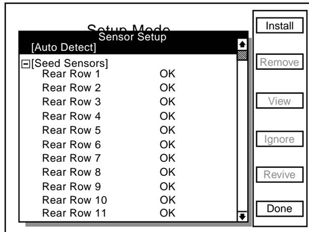
**STEP 6** When "OK" appears behind ALL sensors, press the F6 key next to Done. The "Setup Mode" menu will then appear.
