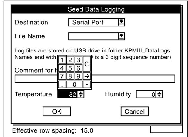
**STEP 9** Use the knob or arrow keys to scroll to the “OK” button and press the knob or Enter key. The display will return to the Setup Mode screen.
