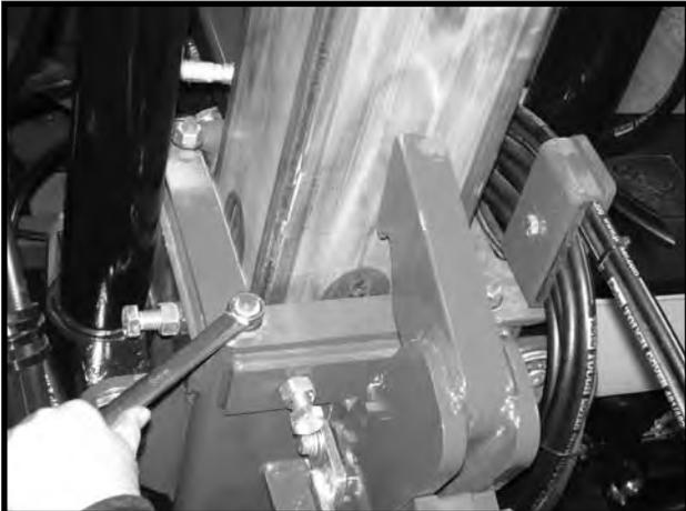
**For pad replacement** (d) As shown below, remove safety hook, disconnect hydraulic hose, remove nut on bulkhead fitting and remove fitting from cap..
