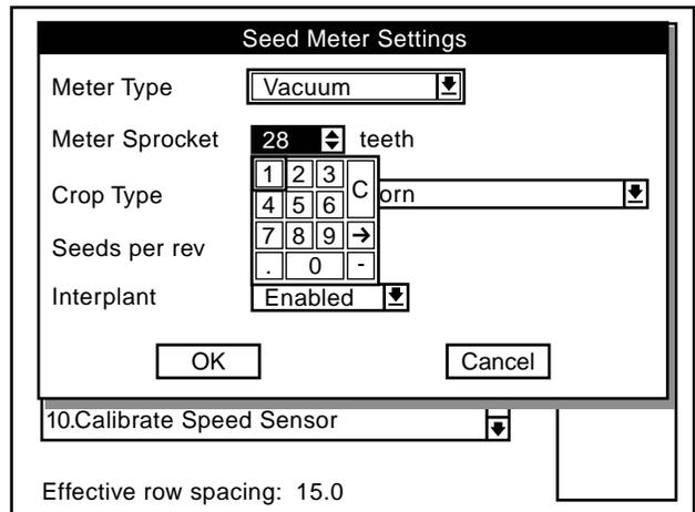
**NOTE:** When Vacuum “Meter Type” is selected “Meter Sprocket” automatically defaults to 28 teeth. To change “Meter Sprocket” select “Meter Sprocket” by turning the knob or using the arrow keys. Press the knob or enter key, a drop down number pad will appear. Turn the knob or use the arrow keys to highlight the first digit of the desired number and press the knob. When the correct number is obtained press the knob or enter key.
