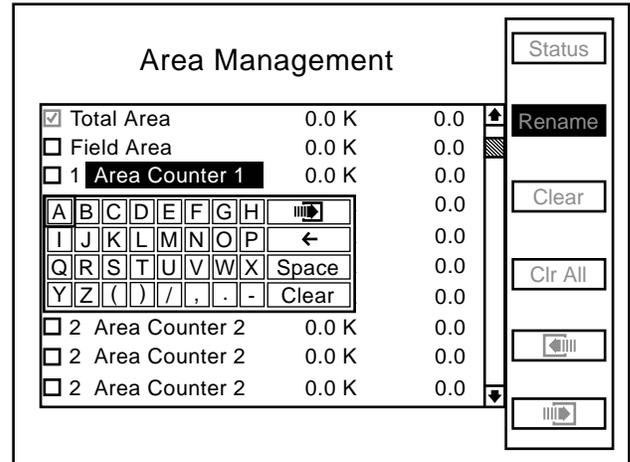
**NOTE: When a key is dimmed it does not perform any operation on the highlighted area counter.**
