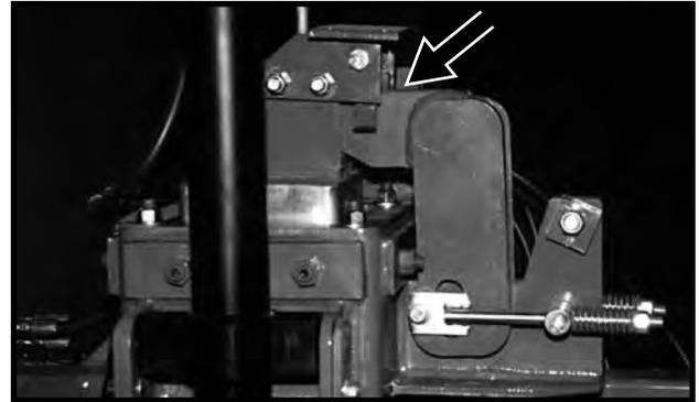
6. Using the hydraulic control, lower the planter onto the safety hook.
