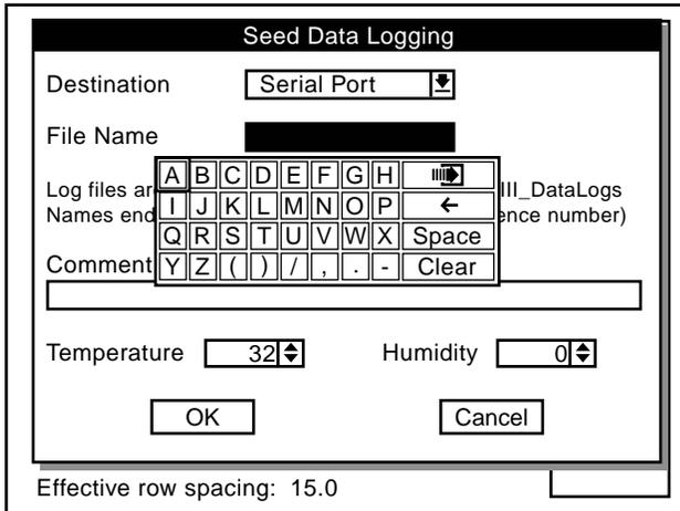
**STEP 6** Use the knob or arrow keys to scroll to the “Comment for file” box. Press the knob or Enter key to display the drop down keyboard. Use the keyboard to enter a Comment for the file then press the Enter key.
