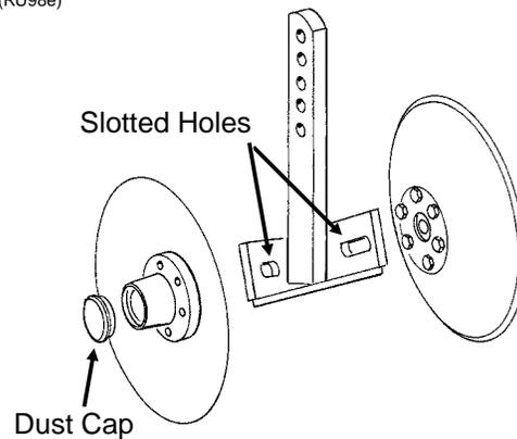
Slotted holes in the support arm where the blades are mounted allow fore and aft adjustment of the disc blades. Blades can be adjusted so the front edges meet or one blade can be moved to the rear and the other to the front of the slot so the cutting edge of one blade overlaps the edge of the other blade. The dust cap must be removed to make these adjustments.
