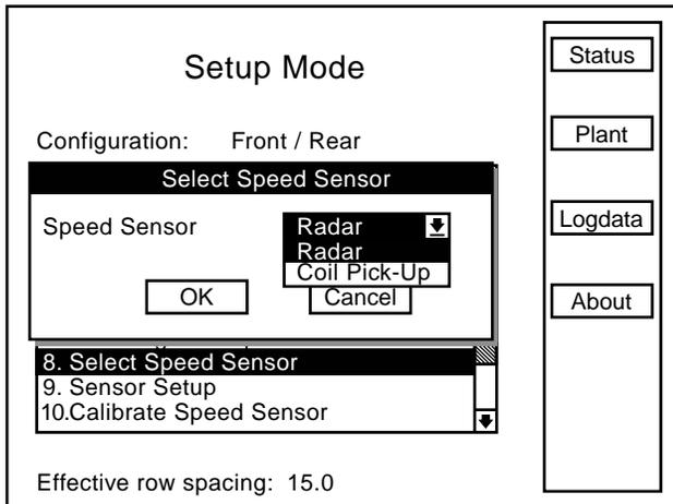
**STEP 3** Turn the knob or use the arrow keys to highlight the “OK” button and press the knob or Enter key to return to the “Setup Mode” screen.
