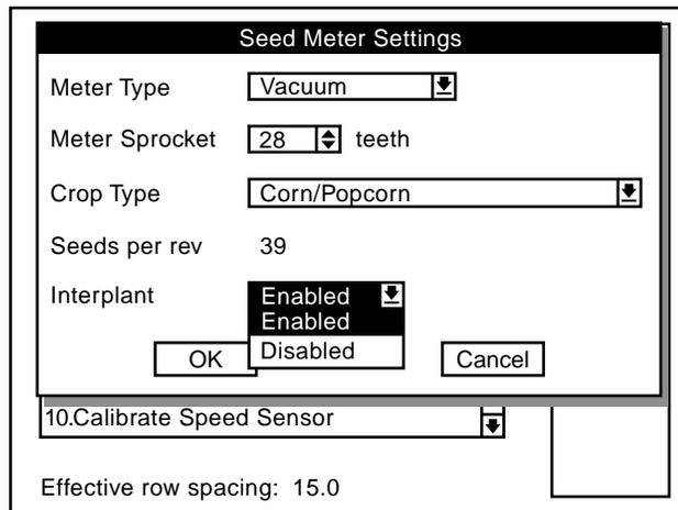
**STEP 6** Turn the knob or use the arrow keys to highlight either “enable” or “disable” and press the knob or Enter key.
