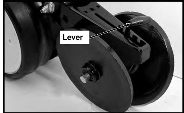
Light soil usually requires less down force at average depth (approximately 2") while heavy soil requires increased down force.
