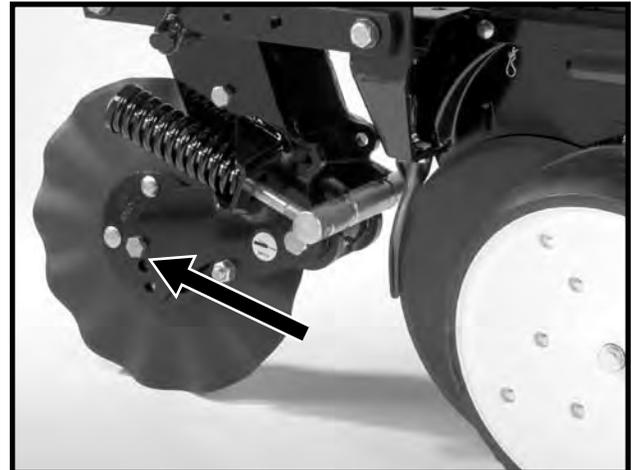
**NOTE: Torque  $\frac{5}{8}$ " spindle hardware to 120 ft. lbs.**
