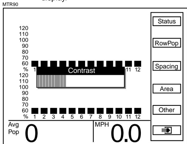
**STEP 2** Use the arrow keys or turn the rotary encoder knob to adjust contrast. The adjustment will be visible on the screen.
