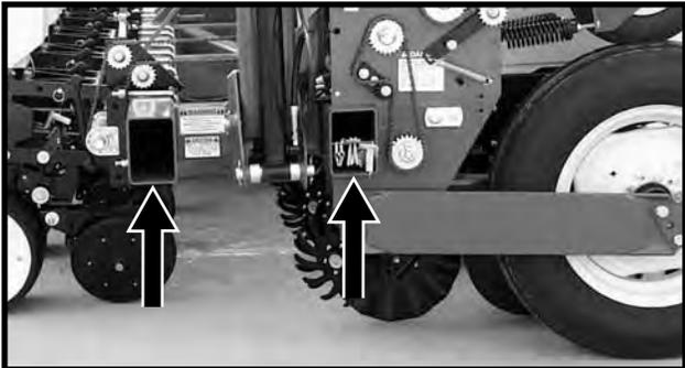
With the planter lowered to correct operating height, check to be sure the frame is level fore and aft. Recheck once planter is in the field.
