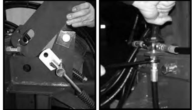
(e) Loosen the four cap mounting nuts and remove pad holder cap. (f) Loosen the pad hex jam nuts, back the pad screws out and remove the four pad holder assemblies as shown below.
