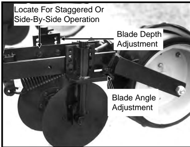
Five sets of holes in each disc bracket allow for 1/2" incremental blade depth adjustment.
