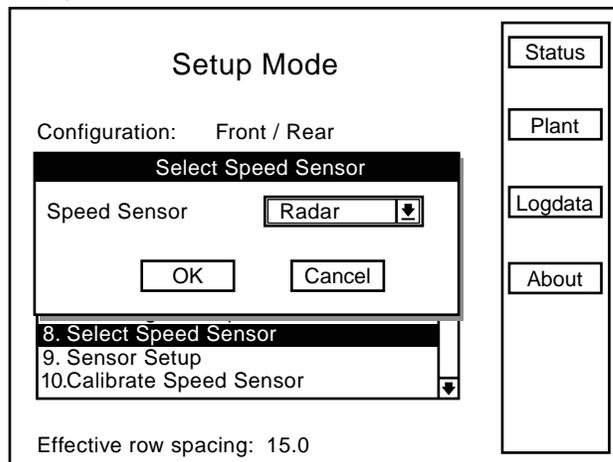
**STEP 4** Press the knob or Enter key to select the “Speed Sensor” field and a drop down menu will appear.
