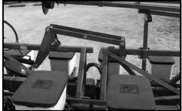
8. Hold the hydraulic lever (to lower planter) to rephase the planter lift cylinders. The length of time it takes to rephase the system may vary due to tractor hydraulic flow and/or oil temperature. Normally 5 to 20 seconds is adequate to rephase the system.
