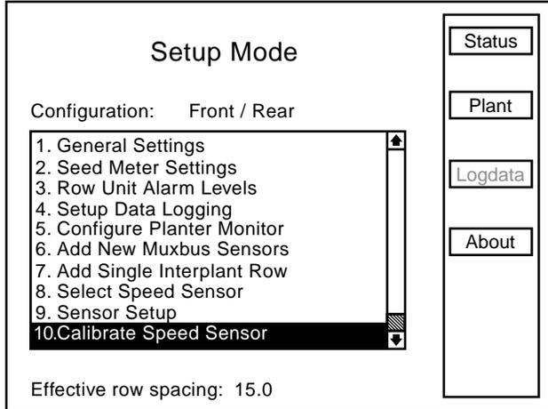
The Distance Pulse Count is used to record how many pulses are generated per mile/kilometer from the ground speed sensor.
