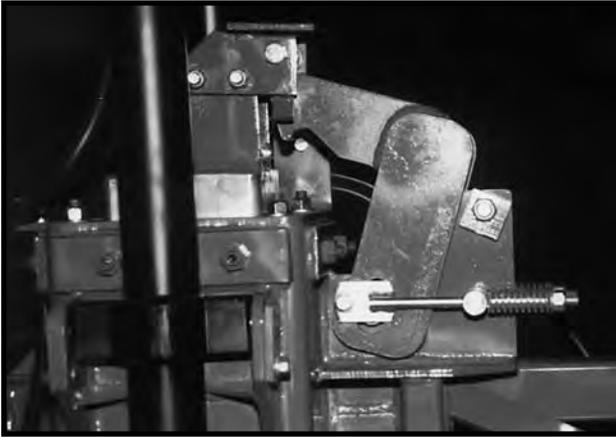
**NOTE:** Raising the planter too high will reset the hook mechanism and the sequence must be repeated.
