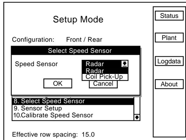
**NOTE: To prevent the configuration from being changed select Cancel, then press the rotary encoder knob, Enter key or ESC key.**
