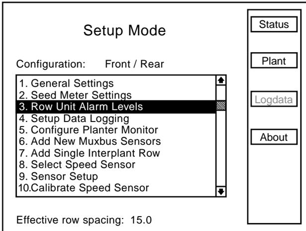
The alarm thresholds can be set for the whole planter, any planter section or individual rows.
