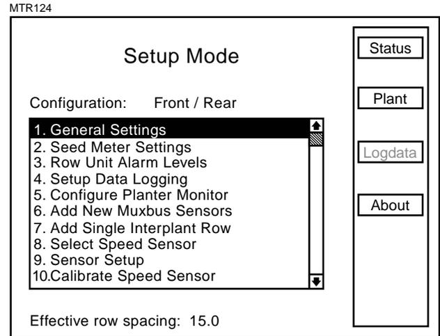
**STEP 9** Turn the knob or use the arrow keys to highlight the “Row Spacing” field. Press the knob or Enter key to make the selection. A drop down number pad will appear. Adjust the row spacing to Interplant spacing by turning the knob or use the arrow keys to highlight the correct value then press the knob to select the number, for numbers containing more than one digit select one digit at a time.
