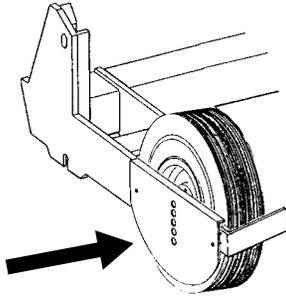
Transport wheel rock guards are designed for use on both sides of each of the four center transport wheels when the planter is used in rocky conditions. Rock guards will help prevent rocks, which can cause damage to the row units, from being picked up by the wheels.
