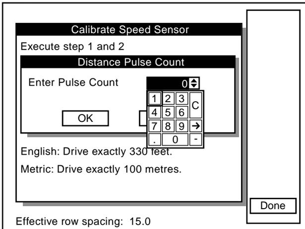
**NOTE: If the Distance Pulse Count number starts to count pulses with the tractor not moving, check radar distance sensor for vibration or other interference.**
