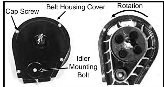
If the belt is being replaced, make sure it is installed to correctly orient the paddles as shown. A diagram molded into the drive sprocket also illustrates the correct orientation.
