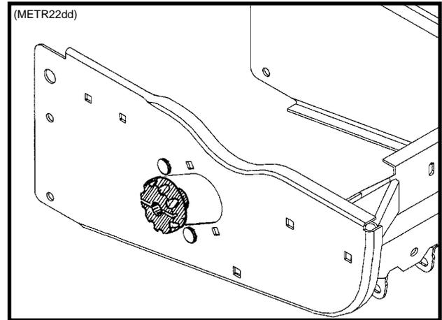
To disengage the drive, turn the knob ¼ turn counter-clockwise. To engage the drive, turn the knob ¼ turn clockwise.
