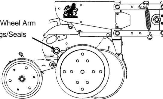
**NOTE: A Gauge Wheel Arm Bushing And Seal Driver Kit (G1K296), for use in bushing and seal replacement, is available through your KINZE® Dealer.**
