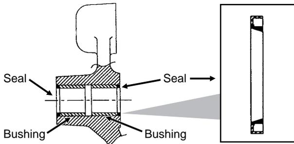
4. Drive/press replacement bushing inside bore of arm to a depth of .125" below flush.
