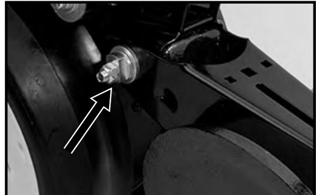
The closing wheels can be installed in two locations either "offset" (to improve residue flow) or "directly" opposite. If set "directly" opposite, the forward installation holes should be used.
