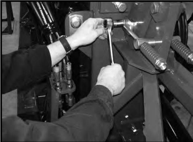
(n) Rotate cam roller against front guide and tighten to 200 ft. lbs. Make sure gap between roller guide and center frame are equal on both sides. (o) Raise planter out of the roller guides and lower back down into roller guides to be sure the roller guides operate smoothly. If not, adjust the rotation cylinder rod as shown below.
