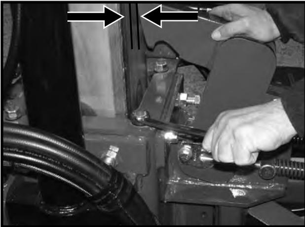
(m) Adjust stop on safety hook. Maximum clearance should be  $\frac{1}{2}$ " and minimum clearance  $\frac{1}{8}$ " as shown above.
