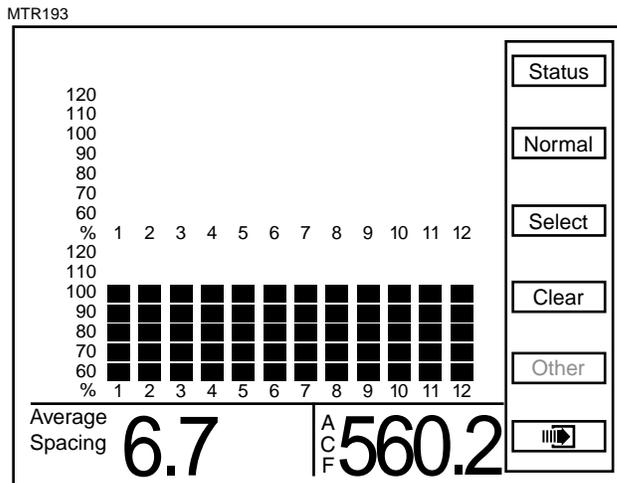
**NOTE:** The abbreviation for the selected area counter will appear in the bottom R.H. corner of the screen. In the above illustration “ACF” stands for Area Counter Field.
