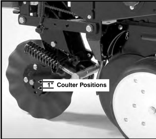
Frame mounted coulters with 1" bubbled, 1" fluted (8 flutes) or 3/4" fluted (13 flutes) blades may be used on pull row units only. **They are not compatible with push row units.**
