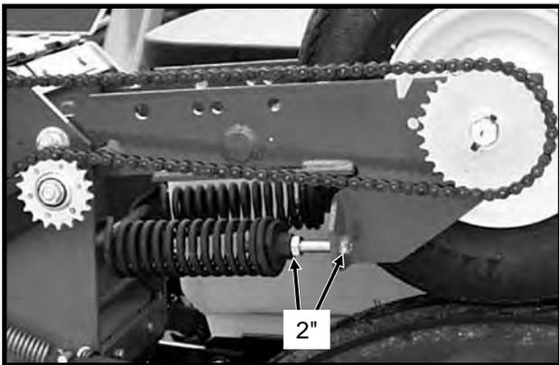
There are two down pressure springs on each contact drive wheel. The down pressure is factory preset and should require no further adjustment.
