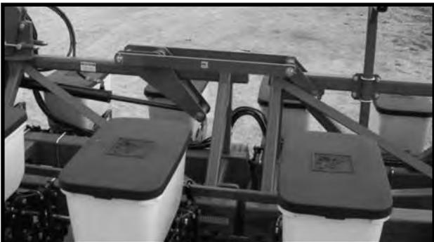
5. Hold the control console switch labeled "RAISE/WING LOCK" in "RAISE" and operate the hydraulic control until the two center lift cylinders are fully extended and the safety hook located at the top of the center section rotates into locking position.
