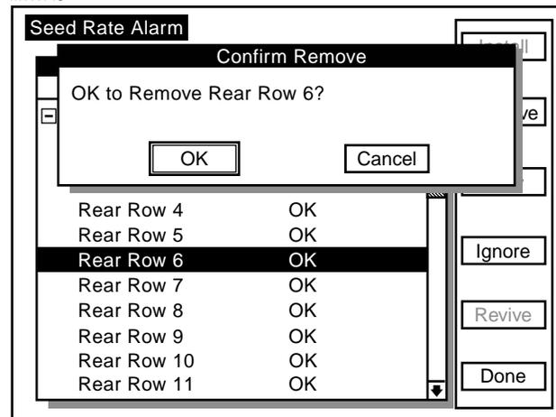
Press the knob or Enter key to confirm removal. The Sensor Setup screen will display "none" next to the row that was removed. Press the F6 key next to "Done". The setup mode screen will appear.
