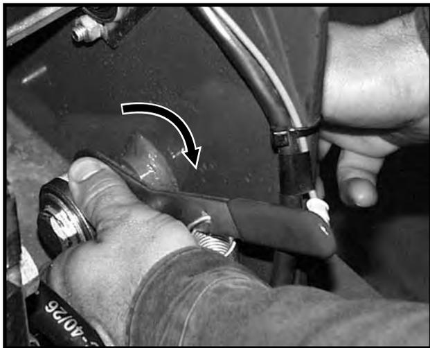
To add chain tension, rotate the chain idler into the chain while rotating the handle to tension idler spring.
