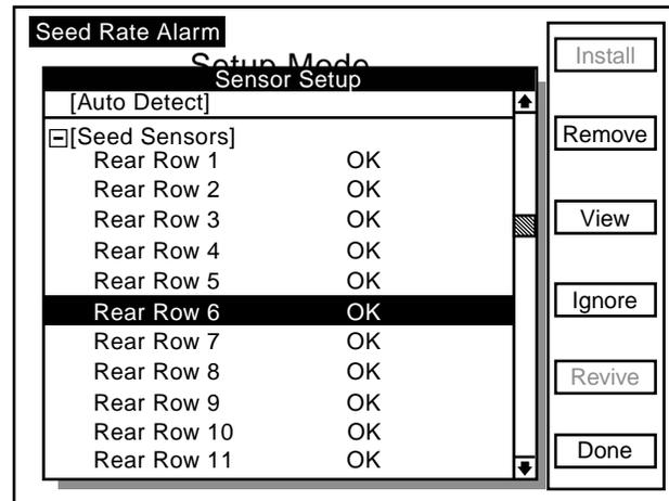
**NOTE:** The only way to remove an alarm is to find the problem and correct it. Alarms are not reported for rows with the seed rate alarm thresholds disabled.
