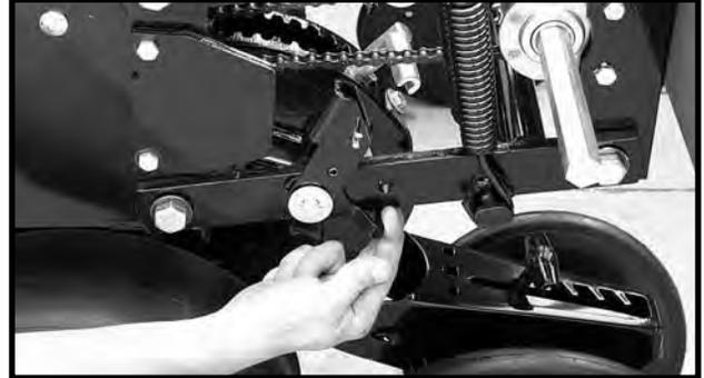
5. Using the lift lever, raise the push row unit to allow the spring loaded lockups to snap into locked position under the row unit stops.
