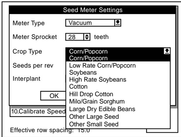
**STEP 4** Turn the knob or use the arrows keys to highlight a crop for planting then press the knob or Enter key. Once crop type is entered, the “Seeds per rev” is set automatically.
