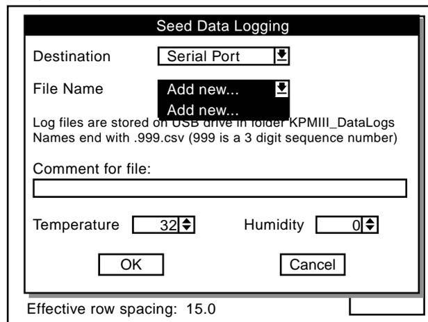
**STEP 4** Select “Add new...” to enter a file name and press the knob or enter key to display a keyboard.
