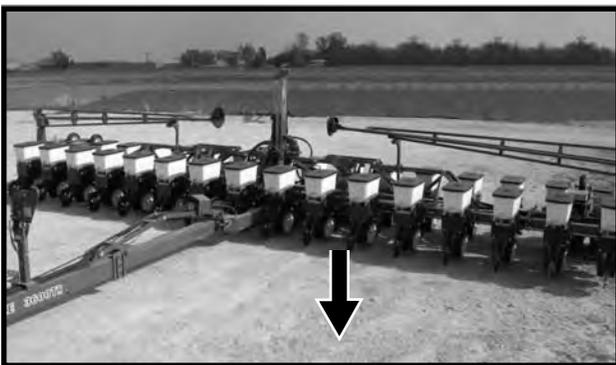
7. Hold the control console switch labeled "RAISE/WING LOCK" in "WING LOCK" and operate the hydraulic lever to release the wing locks.
