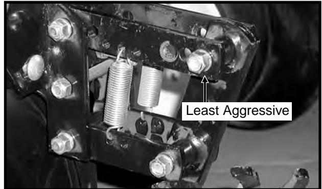
To lock the residue wheel up out of the ground, remove the 1/2" x 5" lockup bolt, raise the residue wheel and install bolt.
