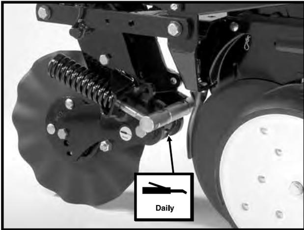
Frame Mounted Coulter - 1 Zerk Per Arm
