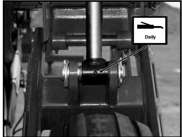
10. Wing Lift Cylinders - 1 Zerk Per Cylinder
