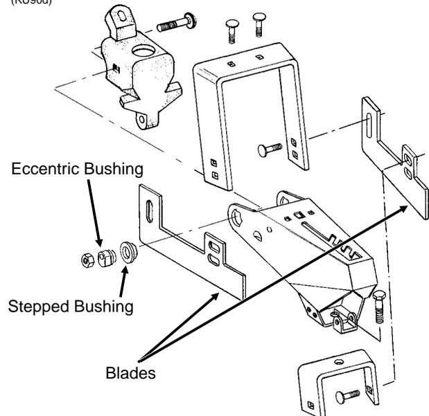
Eccentric bushings allow for lateral adjustment of the drag closing attachment. Using a 3/4" wrench, loosen the hardware which attaches the assembly to the wheel arm stop. Using another 3/4" wrench, turn the eccentric bushings until the drag closing attachment is aligned with the seed trench.
