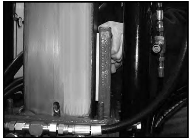
(g) Remove old pads and install new pads. NOTE: Apply a small amount of weather stripping adhesive to hold the pads in place while the pad holder is being reinstalled.
