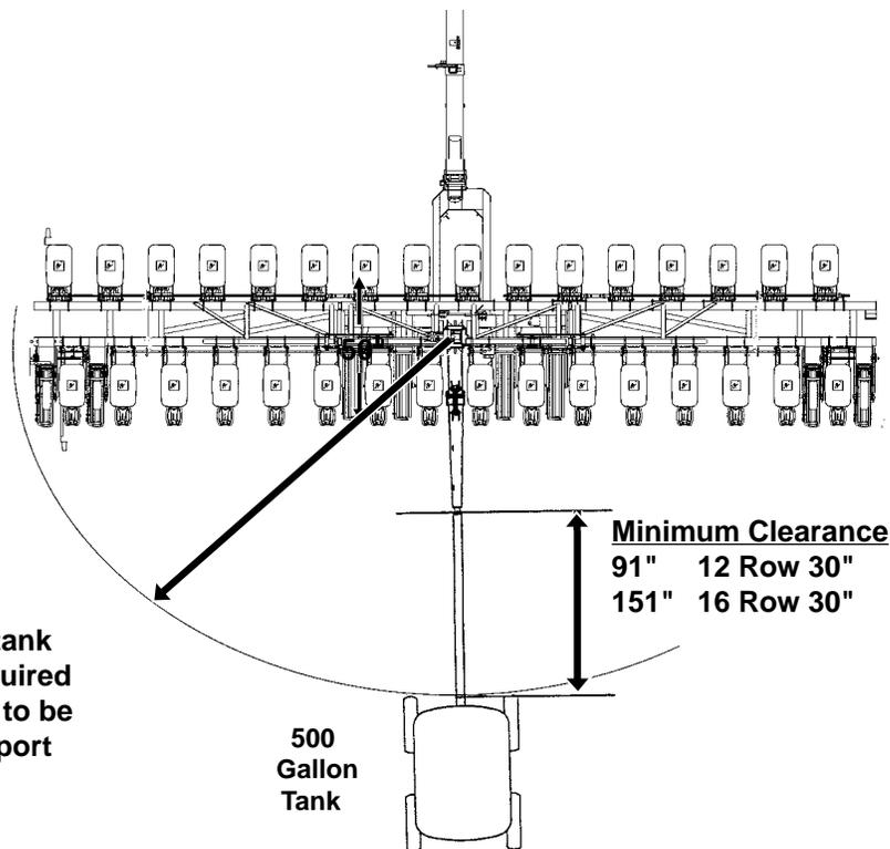
Note minimum tank hitch length required to allow planter to be rotated to transport position.
