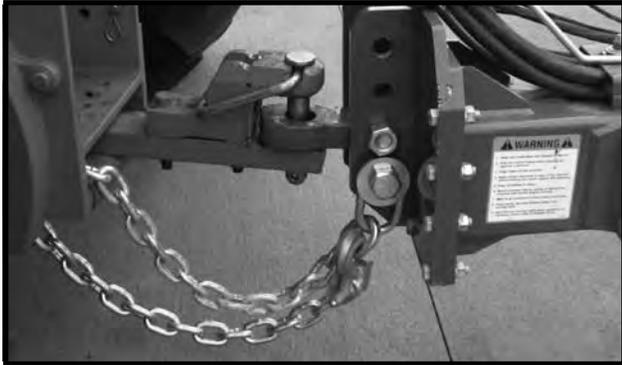
Four holes in the hitch bracket allow the clevis to be raised or lowered. In addition, the clevis may be turned over for a finer adjustment between mounting holes. When installing the clevis mounting bolt, make sure the lock nut is tightened to proper torque setting. (840 ft./lbs.)
