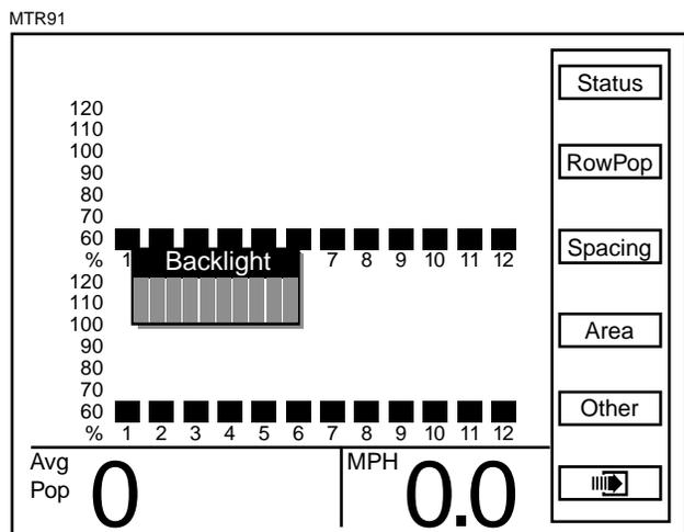
**STEP 5** Use the arrow keys or turn the knob to adjust backlighting. The effect of the adjustment will be visible on the display.
