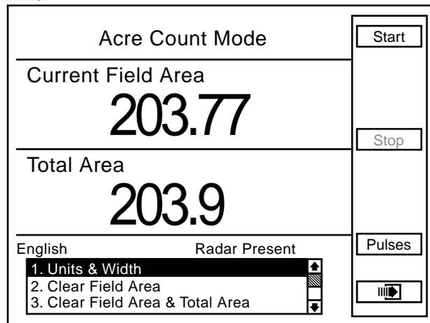
**STEP 4** A box named “Acre Count General Settings” will appear. Highlight the correct units of measure “English” or “Metric” by turning the knob or using the arrow keys. Press the knob or Enter key to make the selection.
