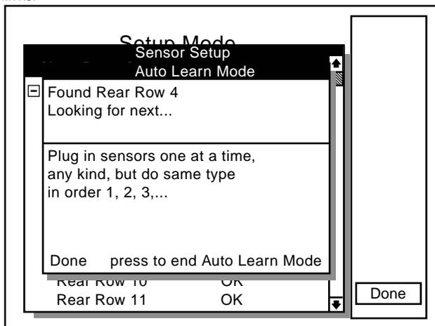
**NOTE:** After each sensor has been installed "OK" will appear after the sensor name on the LCD screen.
