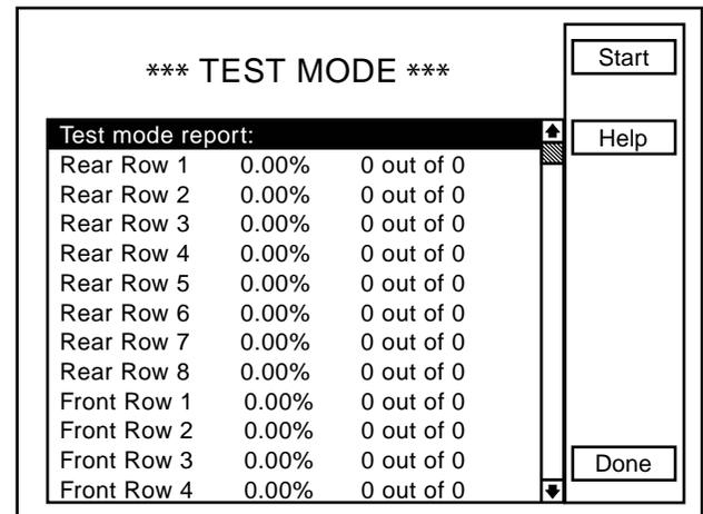
**STEP 6** Begin the test with the tractor stopped. For EdgeVac planters, ensure the vacuum is on and that the seed discs are full.
