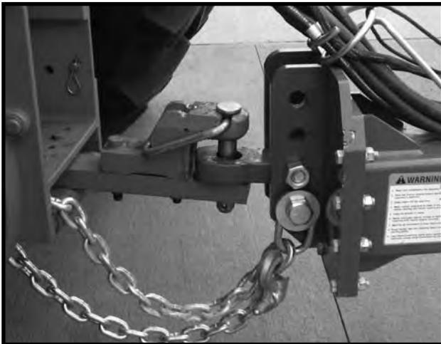
**NOTE: A 2-Point Hitch Option, which converts the planter from drawn to semi-mounted, is available for use with Category 3N or 3 three-point hitch designs. The safety chain is not applicable with the 2-point hitch.**
