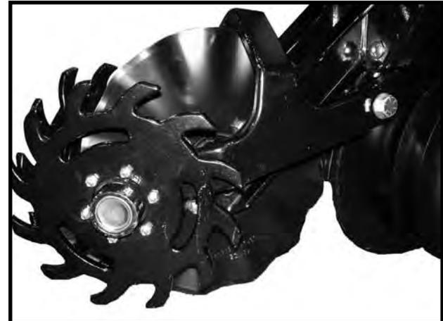
**STYLE B - Used With Style B Row Unit Mounted No Till Couler**
