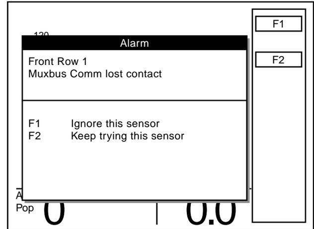
If multiple sensors have lost contact, the message will indicate which sensors have lost contact, see below.
