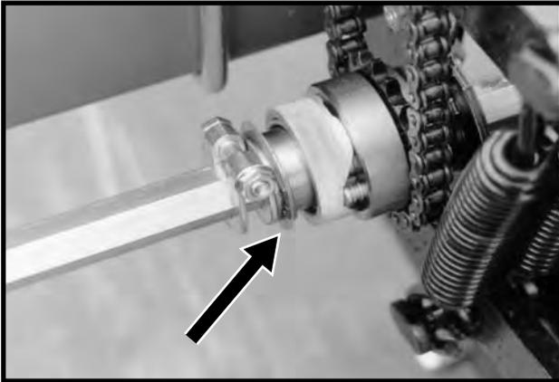
The push row unit clutch sprocket is designed to allow the push row unit drill shaft to be disengaged when only the pull row units are being used.
