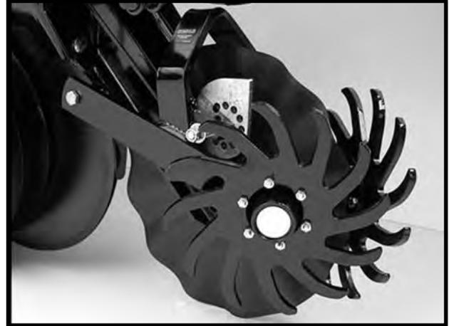
**STYLE A - Used With Style A Row Unit Mounted No Till Couler**
