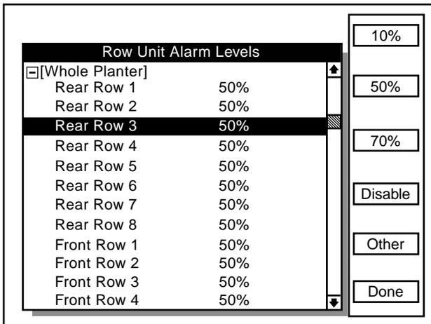
**STEP 2** To set the alarm thresholds for the whole planter, turn the knob or use the arrow keys to highlight the “[Whole Planter]” line. Press the key next to the desired threshold. When the desired threshold has been specified for all row units, press the F6 key next to “Done”.
