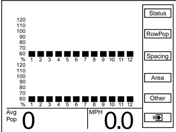
**NOTE:** The Planter Configuration screen displays the planter rows as programmed into the KPM III software. The above screen shows 12 front (Interplant®) rows and 12 rear rows. If the KPM III were programmed for 8 front (Interplant®) rows and 8 rear rows the screen would display 8 front and 8 rear rows.
