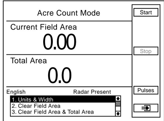
• To Clear Both Field Area And Total Area. Highlight “Clear Field Area & Total Area” and press the knob or Enter key. A note will appear to verify the decision to reset the field area and the total area to zero. Highlight “OK” and press the knob or Enter key to clear the field. Highlight “Cancel” and press the knob or Enter key to retain the current field values.
