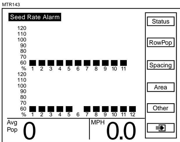
If the sensor is detecting no seed flow it will display which row is not functioning. The alarm may be caused by a mechanical problem reducing seed flow or an electrical problem causing an incorrect seed count.
