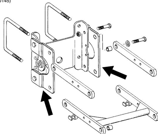
Row unit extension brackets are required on the 4 center pull row units if the Model 3600TR planter is equipped with coulter mounted residue wheels. The brackets extend the row units rearward 4" to provide required clearance.
