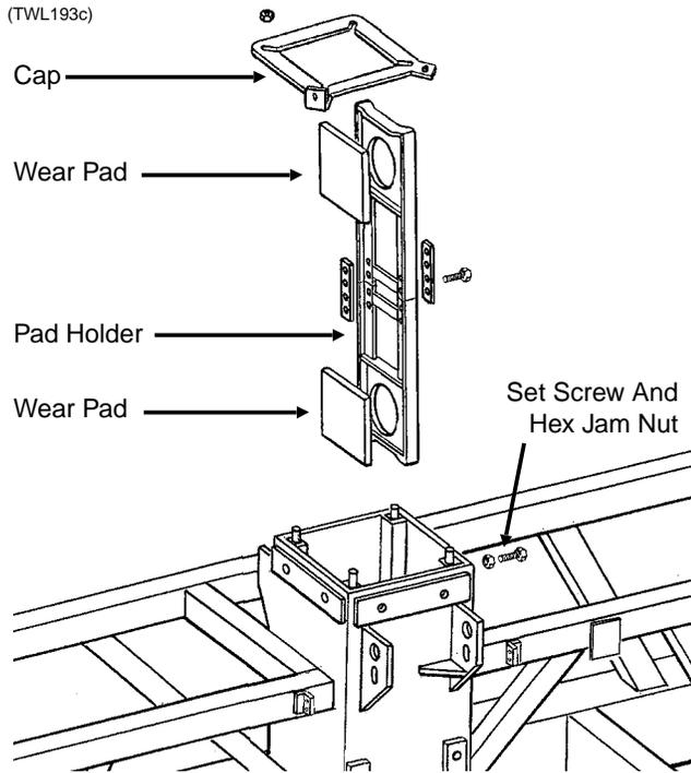
The center section of the planter is constructed around a steel tubular frame with four wear pad assemblies that ride against a stainless steel clad center post. Each wear pad assembly includes a pad holder and two wear pads. The wear pads are held by the pad holder and locked in place by  $\frac{3}{4}$ " set screws and hex jam nuts.
