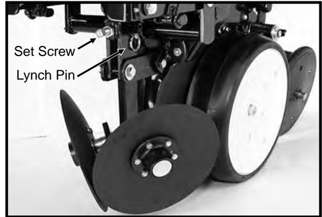
Vertical adjustment in 1/8" increments is possible by removing the lynch pin which secures the vertical support arm and moving the support arm up or down as required. Reinstall lynch pin. Finer adjustment can be attained by removing the lynch pin and using the 5/8" x 2 1/4" set screw to clamp the support arm in the required position.
