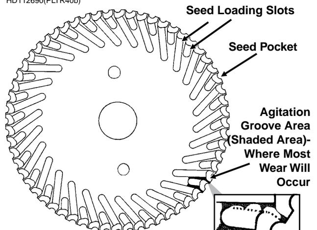
Most wear on the seed disc will be found in the agitation groove area (area between the seed loading slots). Wear will affect planting accuracy at high RPM. To measure for wear, lay a straight edge across the surface of the disc and measure the gap between the disc (at the agitation groove area) and the straight edge. If the agitation groove areas are worn in excess of .030" and accuracy starts to drop off at higher meter RPM, the seed disc should be replaced.
