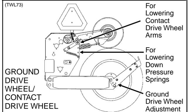
When the planter has been fully loaded with seed, granular chemicals, fertilizer, etc.; a field check should be made to be sure the wings are level with the center frame. If the wings are not level with the center frame, the drive wheels and/or transport wheels can be raised or lowered in the wheel arms to increase or decrease planter toolbar height. Hitch height should be raised accordingly to ensure level operation.
