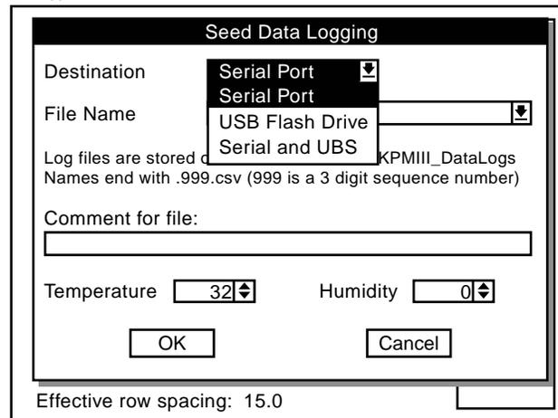
**STEP 3** Use the knob or arrow keys to highlight the “File Name” box. Press the knob or Enter key and a drop down list of the files will be displayed. Select “Add new...” to enter a file name and press the knob or enter key to display a keyboard.
