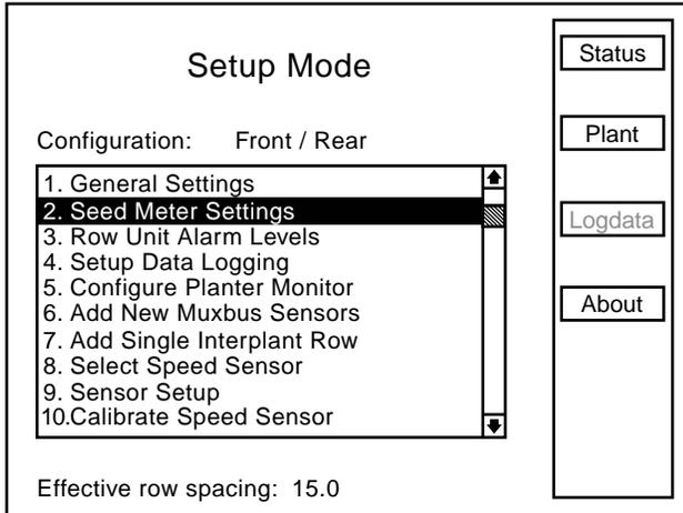
**STEP 2** Select meter type by highlighting “Meter Type” and pressing the knob or Enter key, then highlight “Mechanical” or “Vacuum” and press the knob or enter key.
