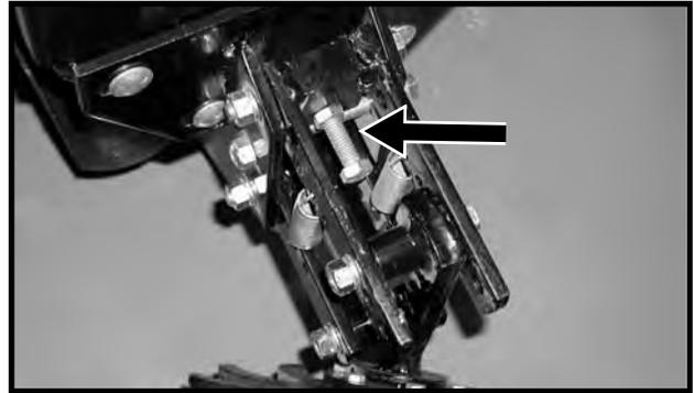
A full threaded bolt and jam nut located on the upper link allows maximum depth to be set for loose soil conditions. Initial setting should be 1 3/4" above the depth of the row unit double disc opener.
