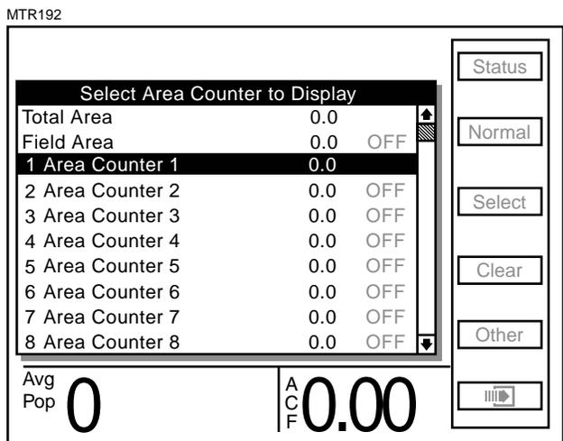
**STEP 3** Use the arrow keys to highlight the desired area counter to be displayed.
