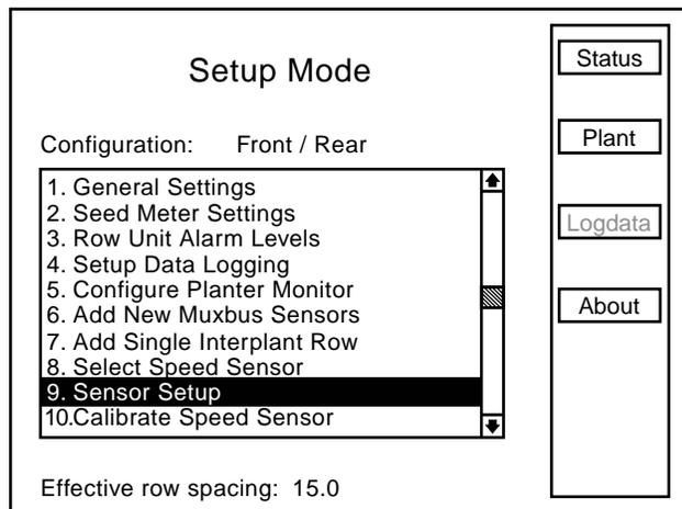
**STEP 3** Turn the knob or use the arrow keys to highlight “8. Select Speed Sensor” and press the knob or Enter key.
