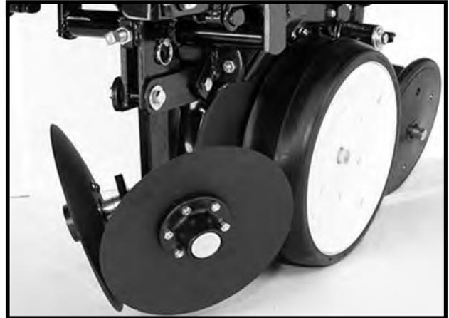
Lubricate the bushings in the support arm and mounting bracket at the frequency indicated in the Lubrication Section of this manual. Using a torque wrench, check each bolt for proper torque. If the bolt is loose, it should be removed and the bushing inspected for cracks and wear. Replace bushings as necessary. **Only hardened flat washers should be used. Replace damaged flat washers with proper part. Torque cap screws to 57 ft. lbs.**
