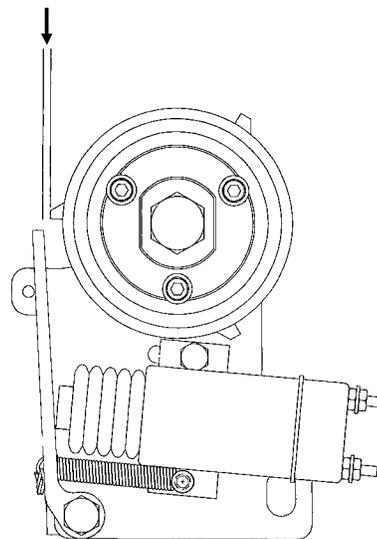
**NOTE: To adjust gap between actuator arm and stop, loosen nut on mounting pin and move pin in slot until there is  $\frac{1}{8}$ " ( $\pm \frac{1}{32}$ ") gap between arm and stop on stop collar. Retighten nut.**
