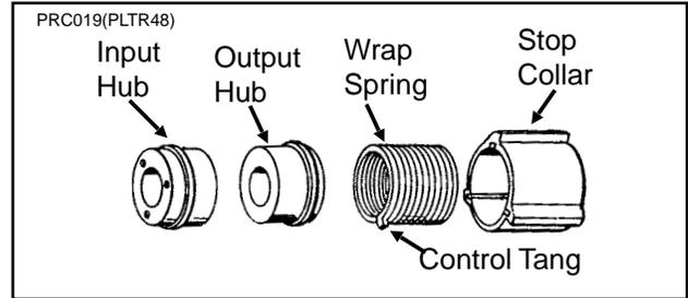
The point row clutch consists of a wrap spring riding on an input hub and an output hub. During operation the wrap spring is wrapped tightly over the hubs connecting them in a positive engagement. The greater the force of rotation the tighter the grip of the spring on the hubs.
