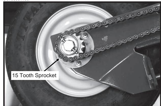
Half rate (2 to 1) drive is recommended only when desired population falls below that shown on planting rate charts. Replace the 30 tooth sprocket on each contact wheel with a 15 tooth sprocket. This will reduce the planter transmission speed and reduce planting and application rates by approximately 50%.
