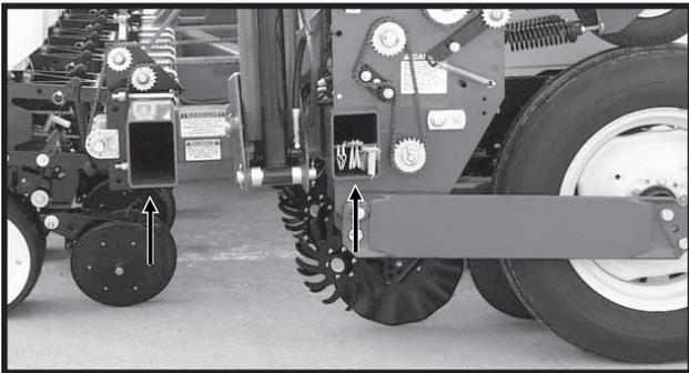
With the planter lowered to proper operating height, check to be sure the frame is level fore and aft. Recheck once planter is in the field.
