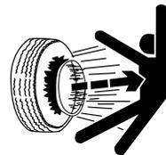
**DANGER:** Rim and tire servicing can be dangerous. Explosive separation of tire and rim parts can cause serious injury or death.
