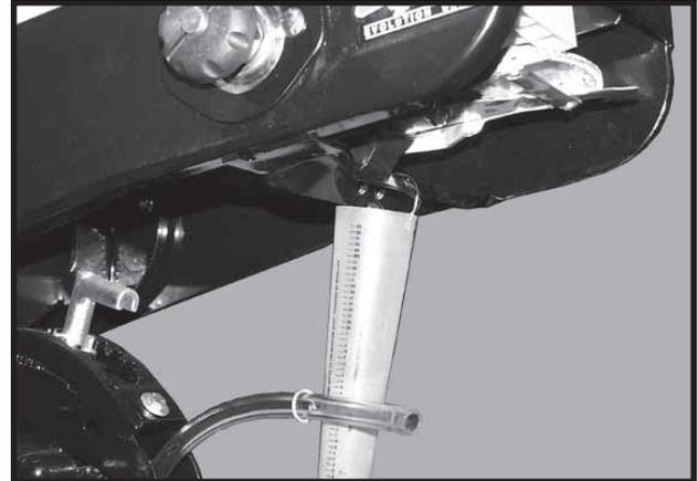
To check, fill insecticide and/or herbicide hoppers. Attach a calibrated vial to each granular chemical meter. Lower the planter and proceed as follows.
