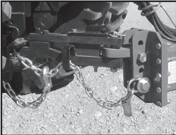
1. Adjust tractor drawbar to 13-17 inches above the ground. Adjust the drawbar so the hitch pin hole is directly below the center line of the PTO shaft. Make sure the drawbar is in a stationary position.
