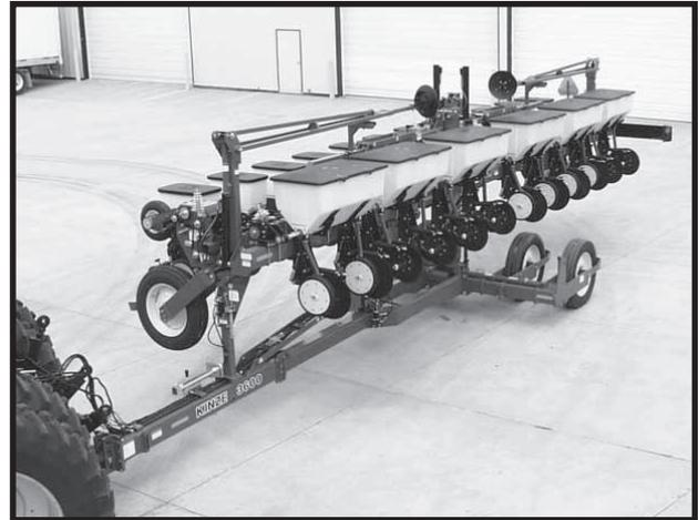
1. With the tongue fully extended and the planter in the raised transport position, remove the tongue safety pin and store it in the storage position.
