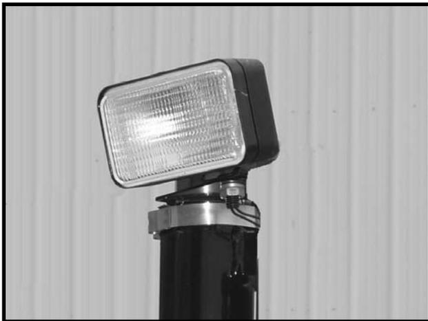
The optional Auxiliary Work Lights Package includes two 50 watt, 3" x 5" halogen flood lamps, hardware to mount lights at the top of one of the center lift cylinders and a wiring harness to plug into the existing planter light harness.
