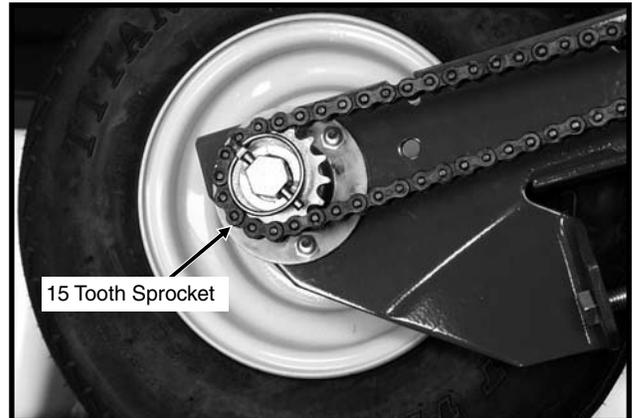
Half rate (2 to 1) drive is recommended only when desired population falls below that shown on planting rate charts. Replace the 30 tooth sprocket on each contact wheel with a 15 tooth sprocket and shorter No. 40 110 pitch chain. This will reduce the planter transmission speed and reduce planting and application rates by approximately 50%.
