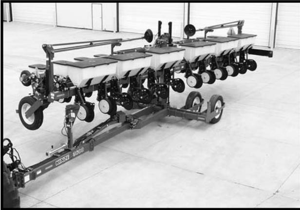
5. Raise the planter 1"-2". The safety hook will release and snap away from the catch pin on the top of the pivot post.
