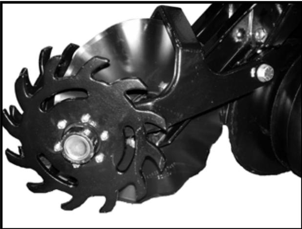
**STYLE B - Used With Style B Row Unit Mounted No Till Coultter**
