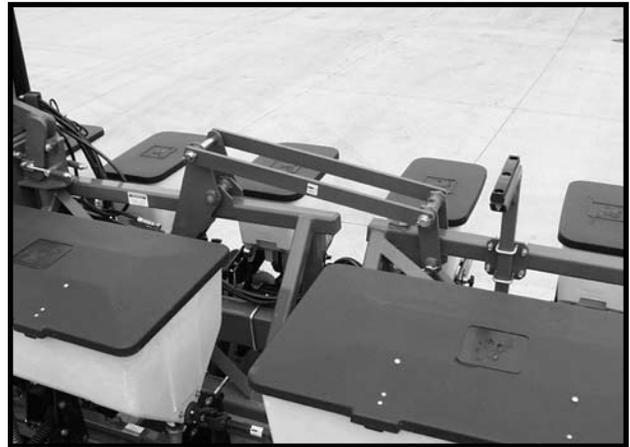
8. Hold the hydraulic lever (to lower planter) to rephase the planter lift cylinders. The length of time it takes to rephase the system may vary due to tractor hydraulic flow and/or oil temperature. Normally 5 to 20 seconds is adequate to rephase the system.
