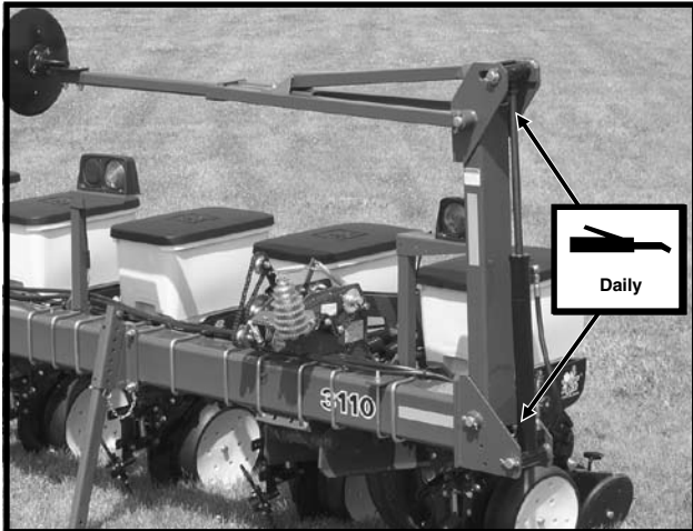
2. Low Profile Row Markers - 2 Zerks Per Assembly
