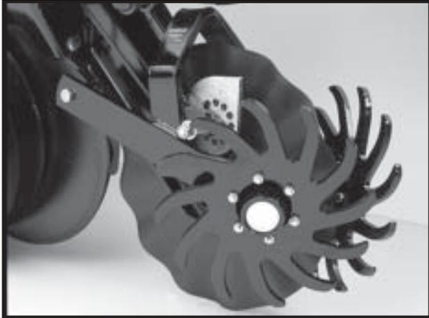
Coulters mounted residue wheels are designed for use on pull row units and push row units. Row unit extension brackets are required on all the pull row units if the planter is equipped with coulters mounted residue wheels and HD single disc fertilizer openers.
