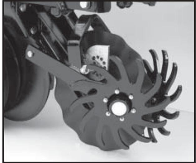
The wheel hubs are equipped with sealed bearings. If bearings sound or feel rough when the wheel is rotated, replace the bearings.
