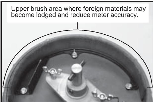
**IMPORTANT:** Replace hopper lids after hoppers are filled to prevent accumulation of dust or dirt in the seed meter which will cause premature wear.
