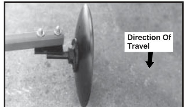
The marker blade is installed so the concave side of the blade is outward to throw dirt away from the grease seals. The spindle assembly is slotted so the hub and blade can be angled to throw more or less dirt. To adjust the hub and spindle, loosen the hardware and move the assembly as required. Tighten bolts to the specified torque.
