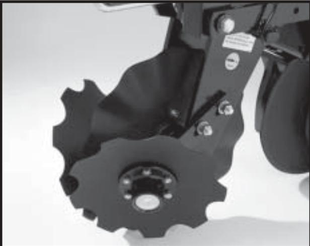
The blade hubs are equipped with sealed bearings. If a bearing sounds or feels rough when the blade is rotated, replace the bearing.
