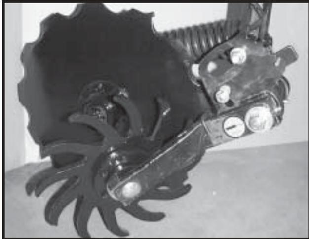
The residue wheel attachment for the notched single disc fertilizer opener is designed for applications where row unit mounted residue wheel attachments cannot be installed. The residue wheel is attached to the notched single disc fertilizer opener using  $\frac{5}{8}$ " x  $7\frac{1}{2}$ " and  $\frac{1}{2}$ " x  $6\frac{1}{2}$ " hardware.
