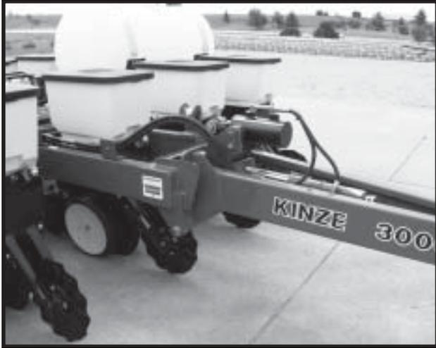
The Interplant® Self-Leveling Hitch Extension is designed to allow the planter to raise level, front to rear, when Interplant® push row units are used.
