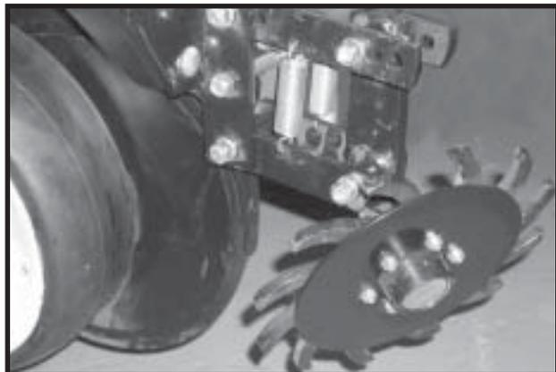
Two adjustable springs on the parallel links on each residue wheel allow for down force adjustment. Position 1 as shown below provides minimum down pressure and position 3 maximum down pressure.
