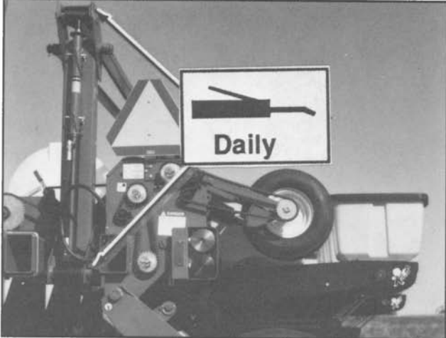
1. Marker Assemblies - 4 Zerks Per Assembly On 8 Row 30, 8 Row Wide & 12 Row 30. 2 Zerks Per Assembly On 12 Row Wide & 16 Row 30.
