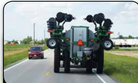
Unique tool-bar design reduces NutriMax applicator folded width to 14'9" for safer transport and space-efficient storage
