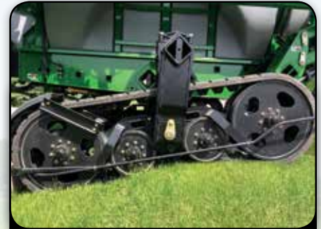
Equalizer tracks with exclusive patent-pending cambering from front-to-rear and side-to-side
